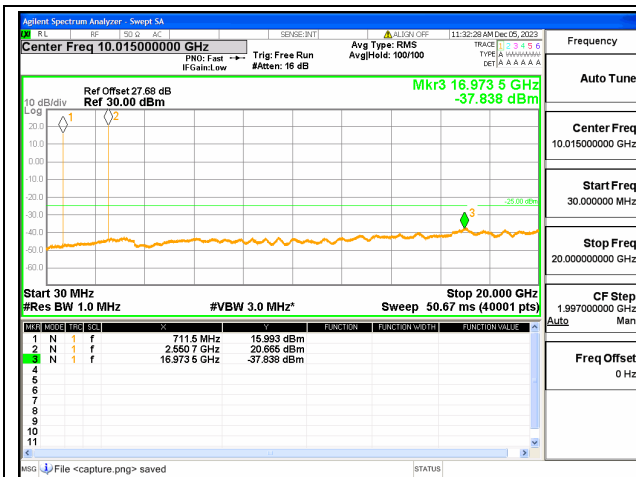
7A-12A-30M-20G / 20+10MHz / QPSK / High+Mid CH / 1@0-1@49
