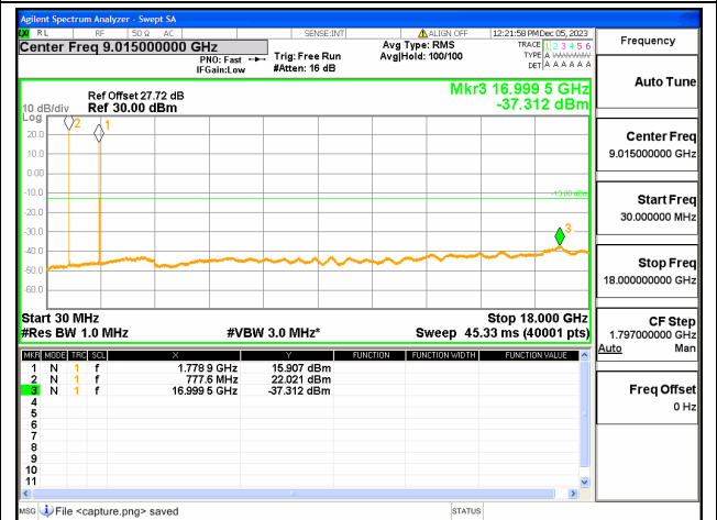
13A-66A / 10+20MHz / QPSK / Mid+High CH / 1@0-1@99
