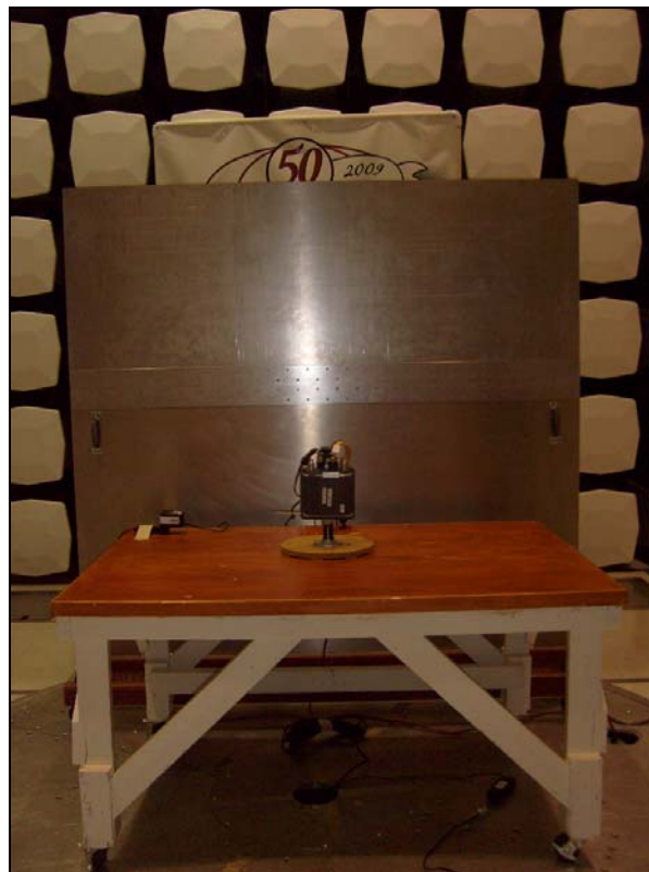
Photograph 3. Conducted Emissions, Test Setup, M25 Radio
