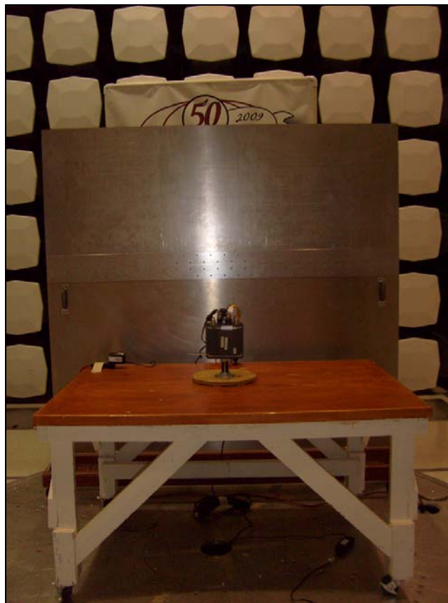
Photograph 6. Conducted Emissions, Test Setup, M5 Radio
