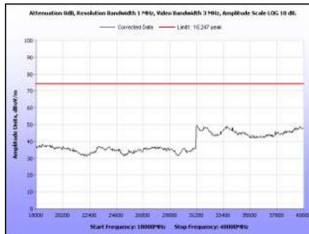
Plot 41. Radiated Spurious Emissions, 5745 MHz, 18 GHz – 40 GHz, Peak, Dish Antenna
