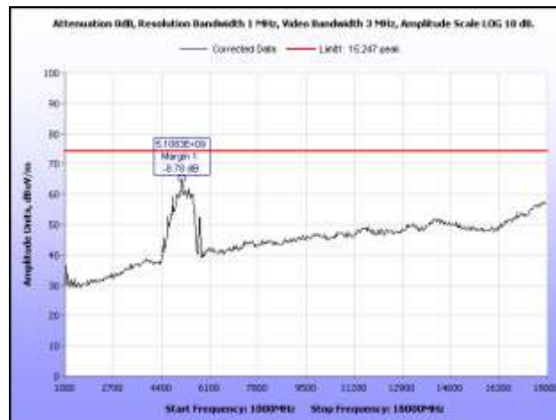
Plot 39. Radiated Spurious Emissions, 5745 MHz, 1 GHz – 18 GHz, Peak, Dish Antenna
