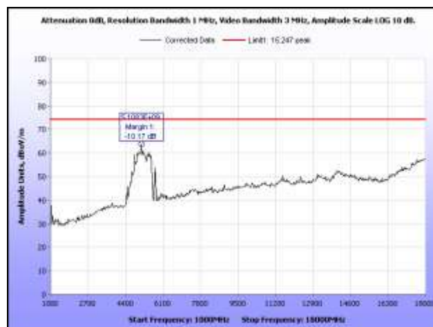
Plot 24. Radiated Spurious Emissions, 5745 MHz, 1 GHz – 18 GHz, Peak, Omni Antenna
