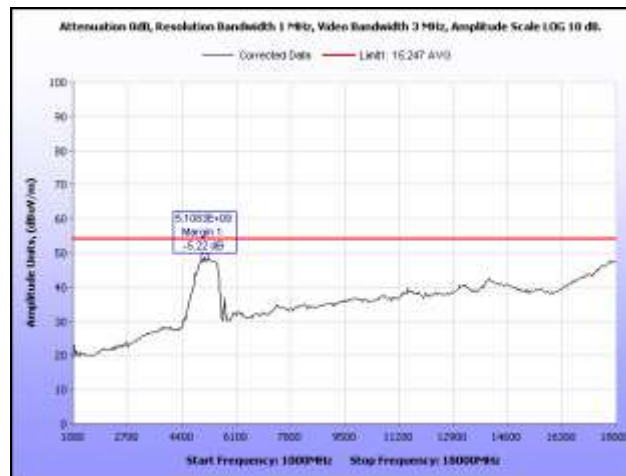
Plot 38. Radiated Spurious Emissions, 5745 MHz, 1 GHz – 18 GHz, Average, Dish Antenna
