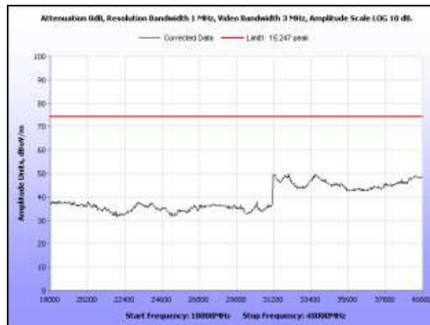
Plot 36. Radiated Spurious Emissions, 5805 MHz, 18 GHz – 40 GHz, Peak, Omni Antenna
