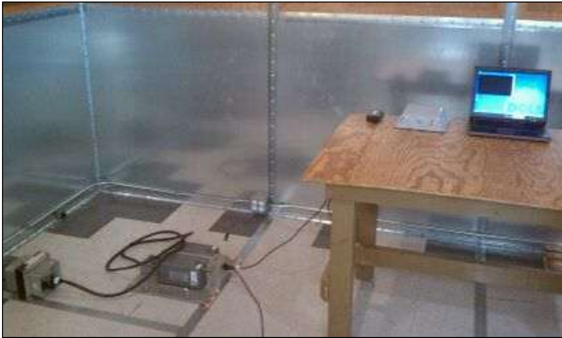
Photograph 2. Conducted Emissions, Test Setup
