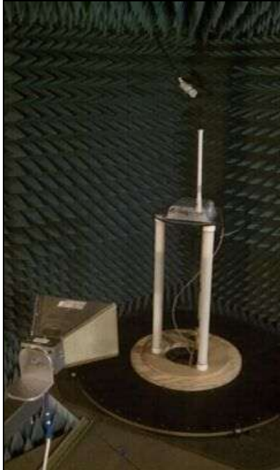
Photograph 4. Radiated Spurious Emissions, Test Setup (1)
