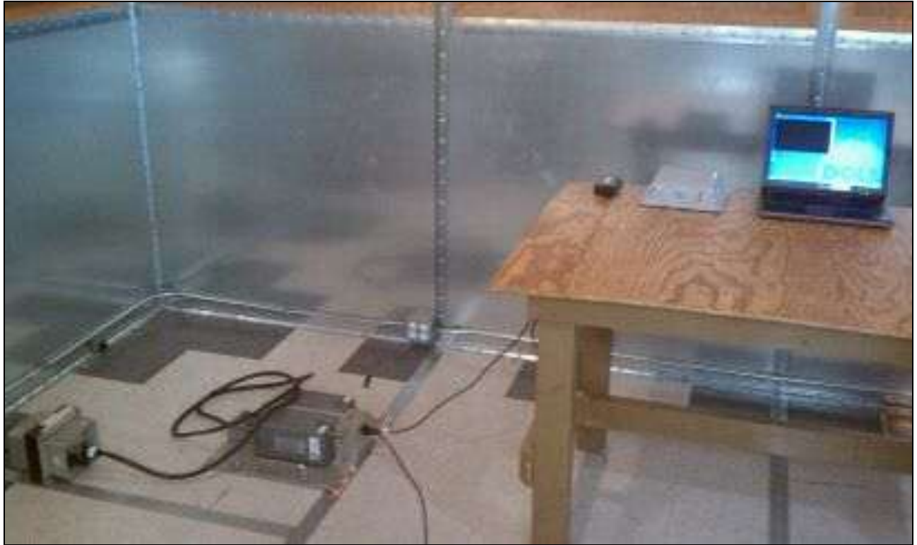
Photograph 2. Conducted Emissions, Test Setup
