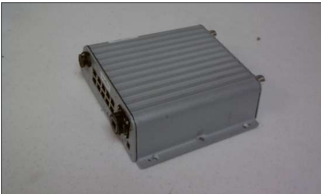
Photograph 1. Deployable Mesh Point Model: ES520 (with Senao Modular Approved Radio)
