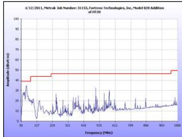
Plot 46. Radiated Spurious Emissions, Mid Channel, 30 MHz – 1 GHz, 5.8 GHz, HT20
