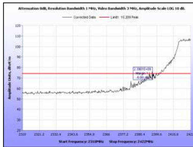
Plot 92. Radiated Restricted Band Edge, 2432 MHz, Peak, HT40
