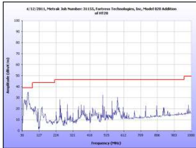
Plot 62. Radiated Spurious Emissions, High Channel, 30 MHz – 1 GHz, 2.4 GHz, HT40
