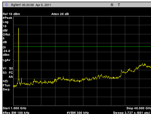
Plot 104. Conducted Spurious Emissions, High Channel, 1 GHz – 40 GHz, 2.4 GHz, HT20
