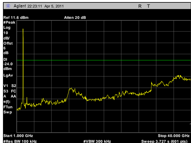
Plot 116. Conducted Spurious Emissions, High Channel, 1 GHz – 40 GHz, 2.4 GHz, HT40
