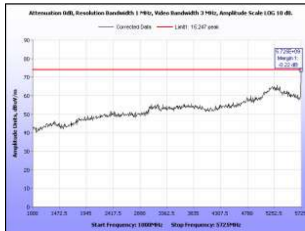
Plot 42. Radiated Spurious Emissions, Low Channel, 1 GHz – 5.725 GHz, Peak, 5.8 GHz, HT20
