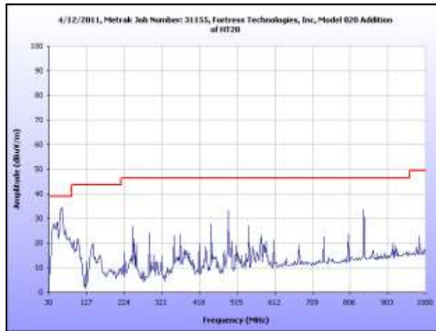
Plot 38. Radiated Spurious Emissions, High Channel, 30 MHz – 1 GHz, 2.4 GHz, HT20
