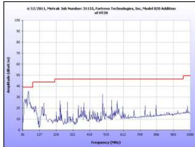
Plot 52. Radiated Spurious Emissions, High Channel, 30 MHz – 1 GHz, 5.8 GHz, HT20
