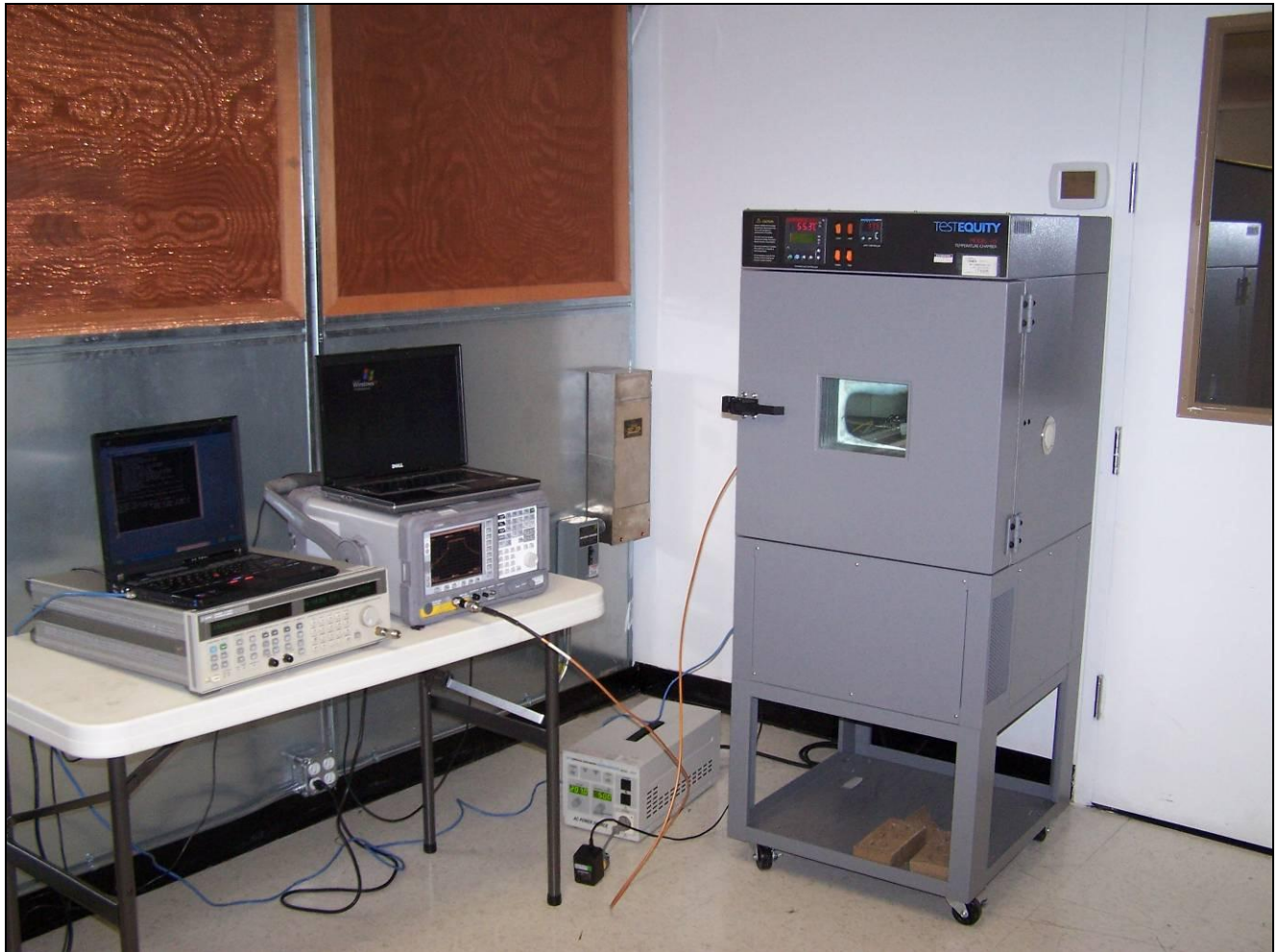
Photograph 11. Frequency Stability, Test Setup, M5 Radio
