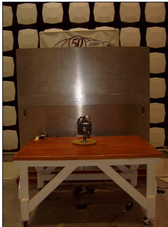
Photograph 8. Conducted Emissions, Test Setup, M5 Radio
