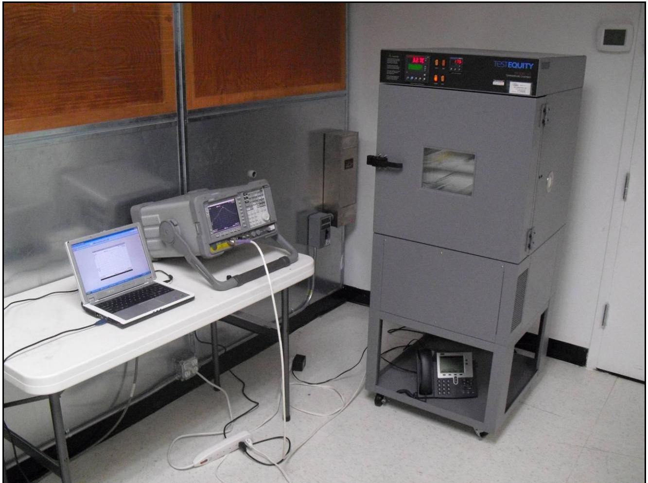
Photograph 6. Frequency Stability, Test Setup, M25 Radio
