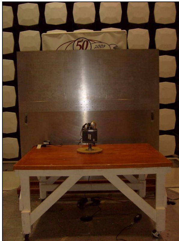
Photograph 3. Conducted Emissions, Test Setup, M25 Radio
