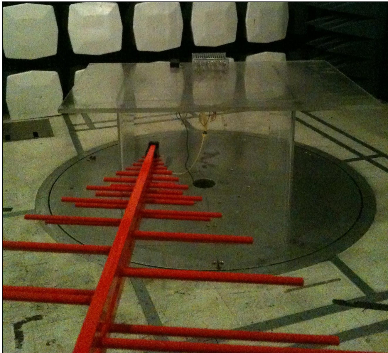
Photograph 3. Radiated Emission, Test Setup
