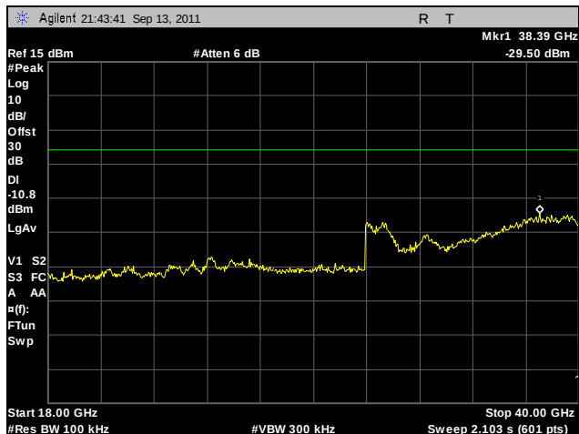
Plot 211. Conducted Spurious Emissions, Low Channel, 802.11a, Port A, 18 GHz – 40 GHz
