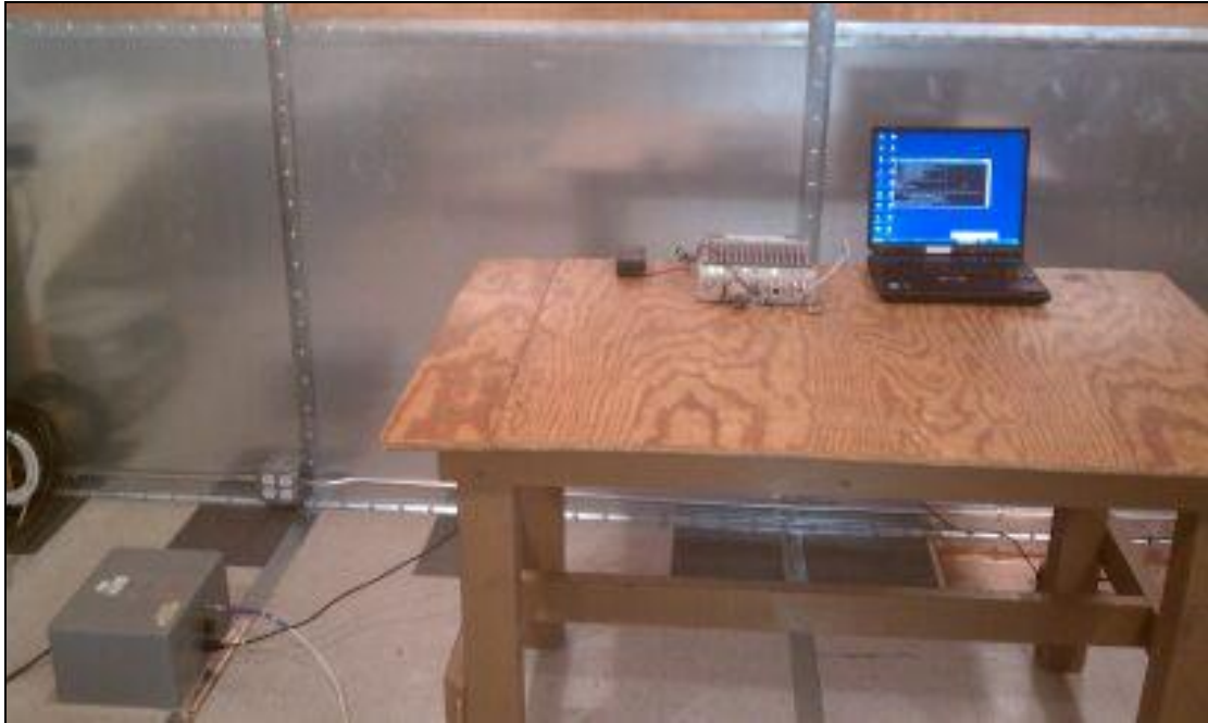
Photograph 4. Conducted Emissions, 15.207(a), Test Setup
