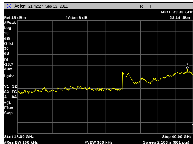
Plot 214. Conducted Spurious Emissions, Mid Channel, 802.11a, Port A, 18 GHz – 40 GHz
