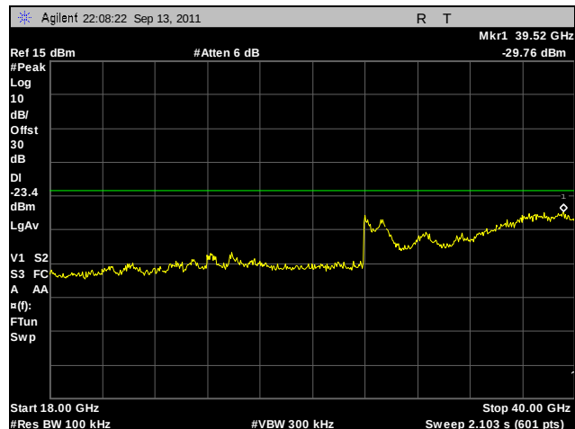
Plot 247. Conducted Spurious Emissions, Low Channel, 802.11n 40 MHz, Port B, 18 GHz – 40 GHz
