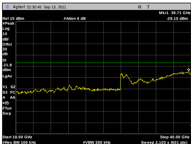
Plot 229. Conducted Spurious Emissions, Low Channel, 802.11n 20 MHz, Port B, 18 GHz – 40 GHz
