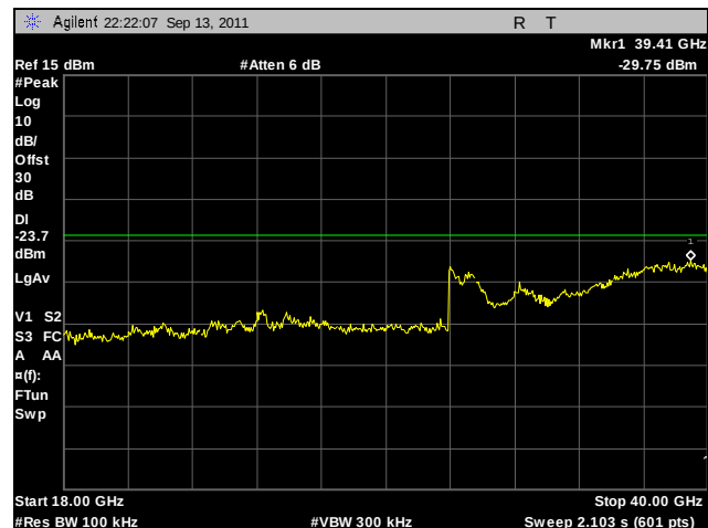
Plot 235. Conducted Spurious Emissions, High Channel, 802.11n 20 MHz, Port B, 18 GHz – 40 GHz
