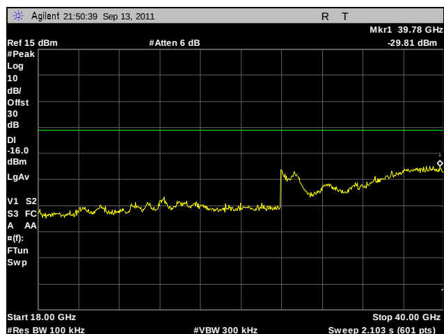
Plot 241. Conducted Spurious Emissions, Mid Channel, 802.11n 40 MHz, Port A, 18 GHz – 40 GHz
