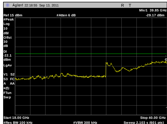
Plot 253. Conducted Spurious Emissions, High Channel, 802.11n 40 MHz, Port B, 18 GHz – 40 GHz
