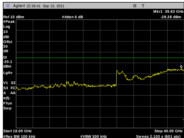
Plot 232. Conducted Spurious Emissions, Mid Channel, 802.11n 20 MHz, Port B, 18 GHz – 40 GHz
