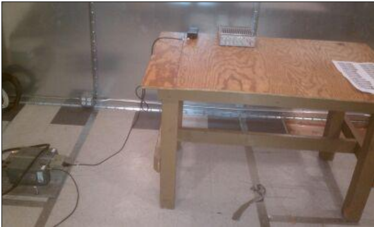
Photograph 2. Conducted Emissions, Test Setup
