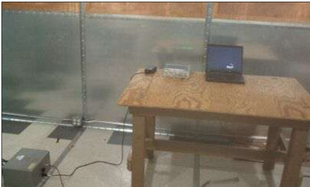
Photograph 1. Conducted Emissions, Test Setup
