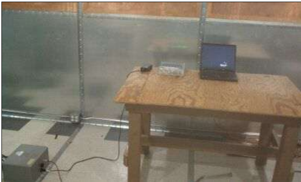
Photograph 3. Conducted Emissions, 15.207(a), Test Setup
