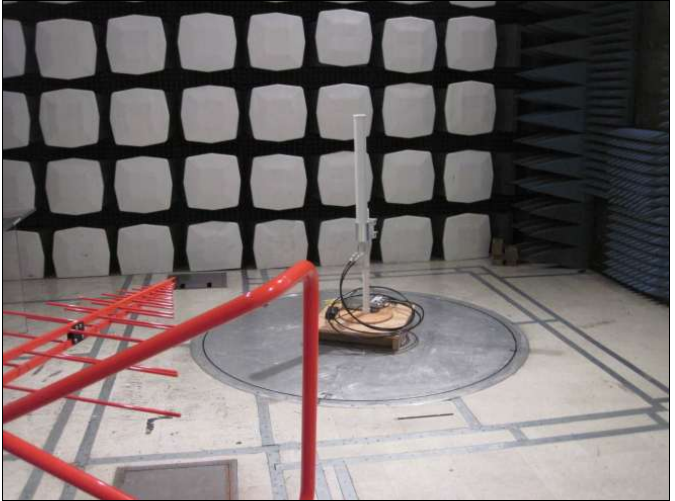
Photograph 2. Radiated Emission, Test Setup
