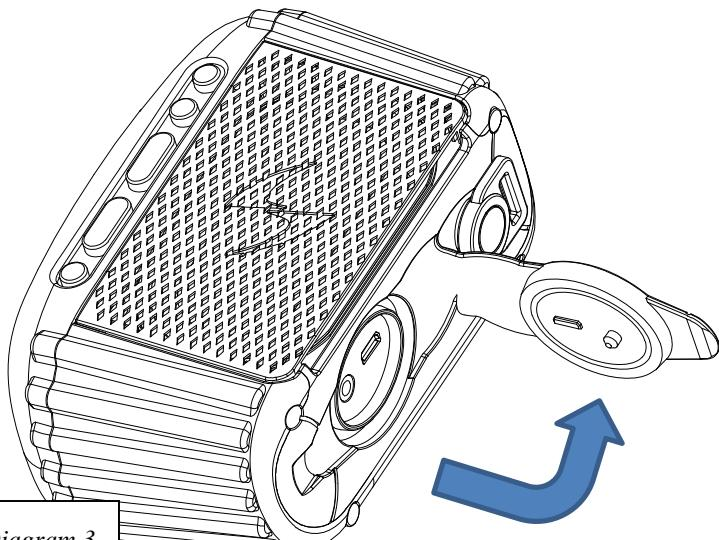
*Diagram 3***RUBBER CAP, USB POWER & AUX-IN CONNECTIONS**
