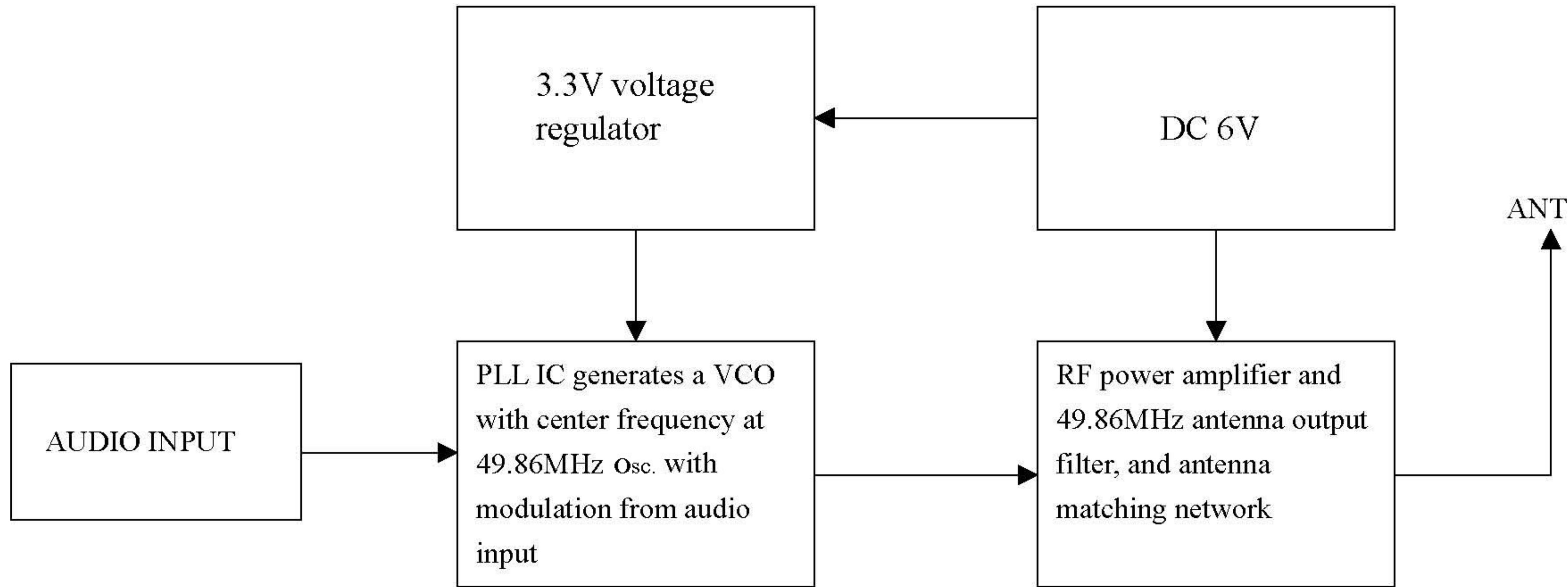
49.86MHz transmitter operation block diagram
