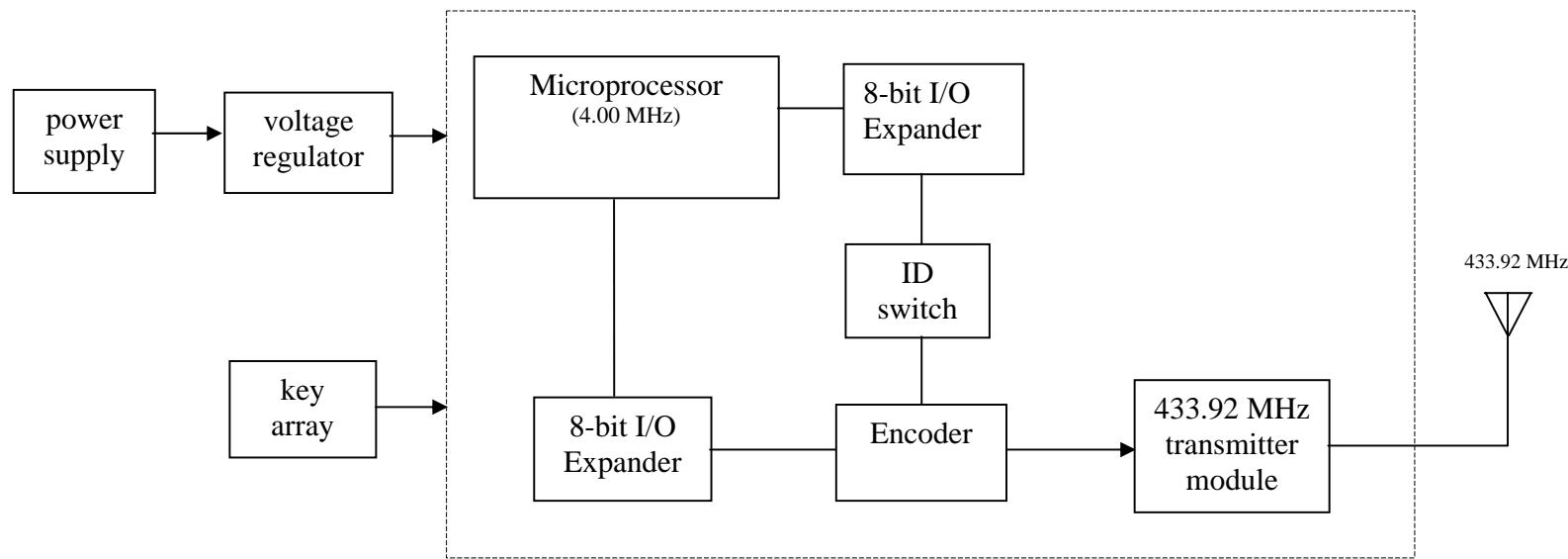
Transmitter block diagram
