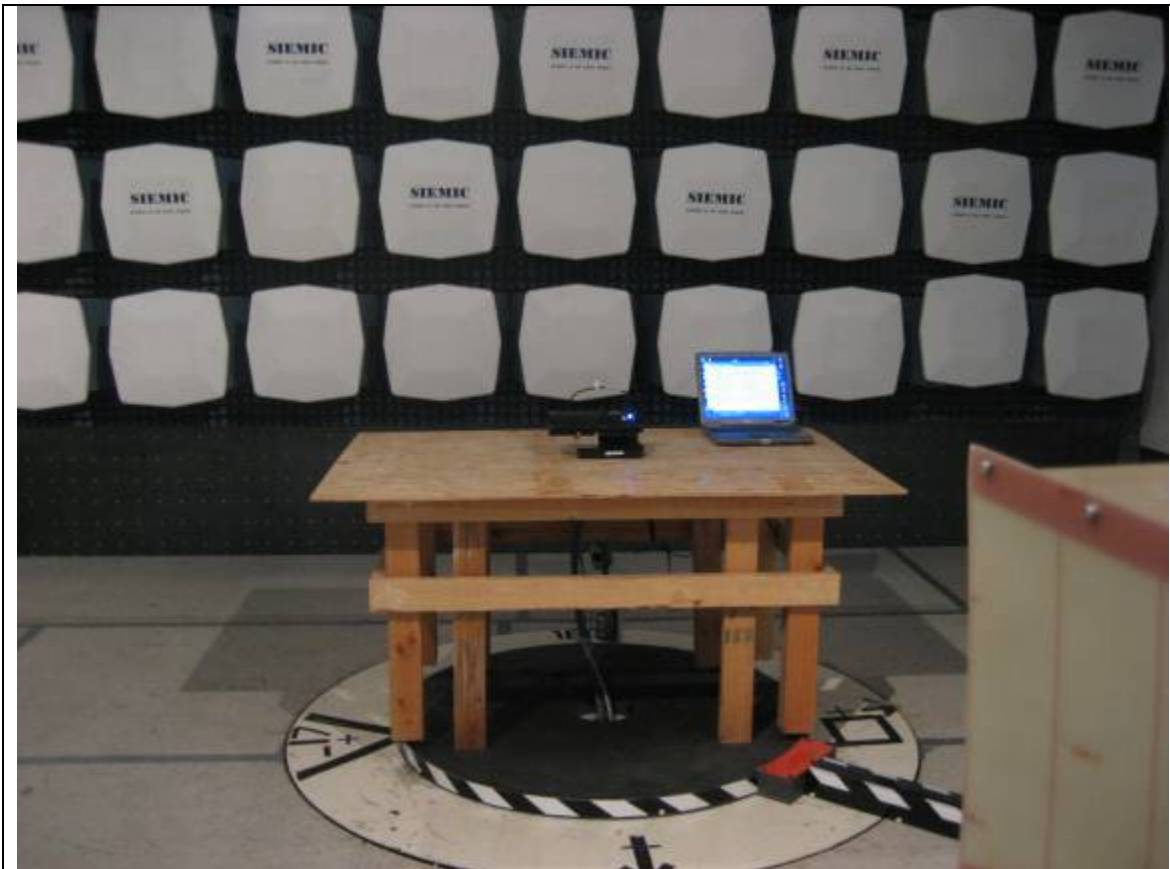
Radiated Emission Test Setup – Front View (>1GHz)
