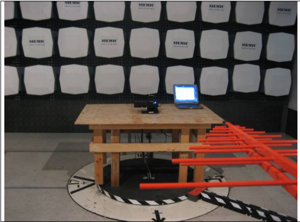
Radiated Emission Test Setup – Front View (<1GHz)
