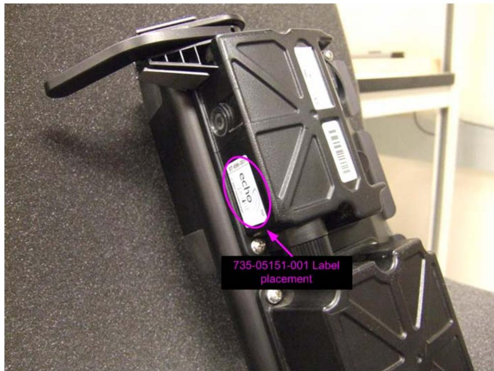
6. Place label 735-05166-001 on Antenna housing sub-assembly as shown:
