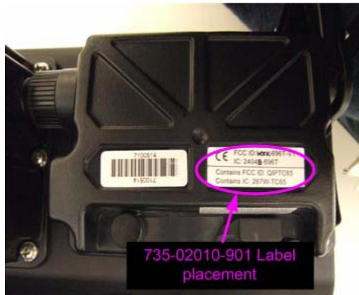
2. Place label 735-04513-001 on Sensor housing sub-assembly as shown:
