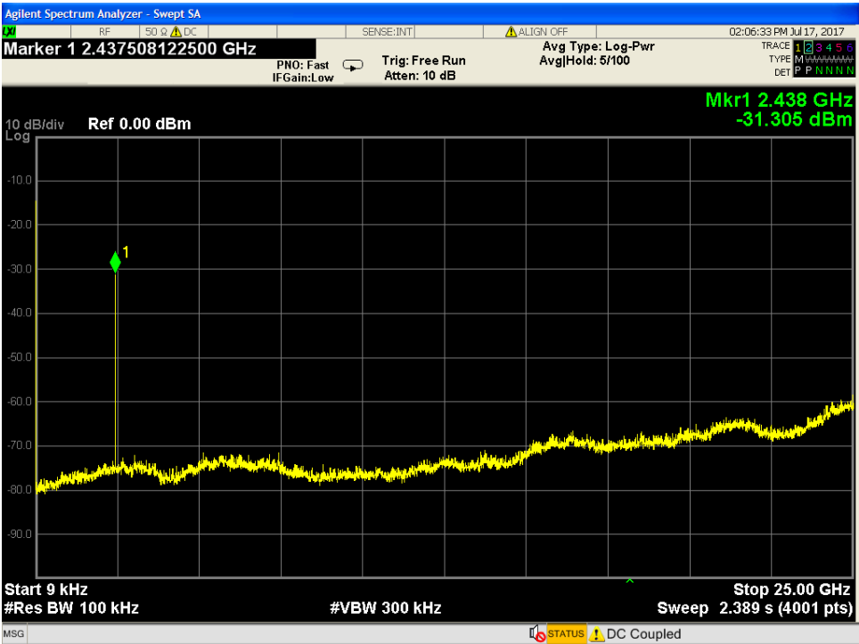
Middle Channel 9 KHz -25GHz Conducted Spurious
