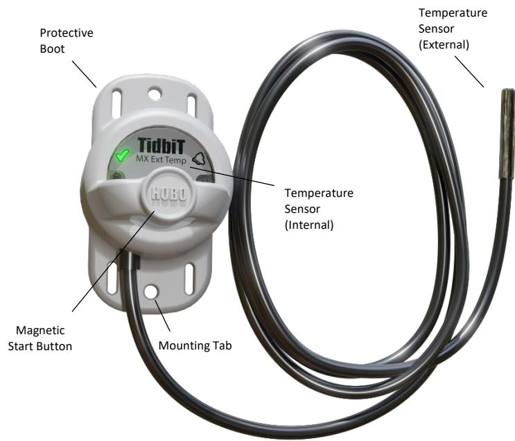
**Protective Boot:** This waterproof cover protects the logger during deployment. It has two mounting tabs and a built-in magnet to use with the logger's internal reed switch (see *Deploying and Mounting the Logger*).
