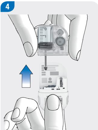
Remove the used reservoir from the pump base.
