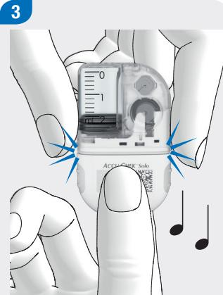
When both components are connected to each other correctly and the battery is activated, the micropump issues the "Start" signal sequence. If this sequence of signals is not issued, check whether the battery is activated and repeat Steps 1 to 3.
