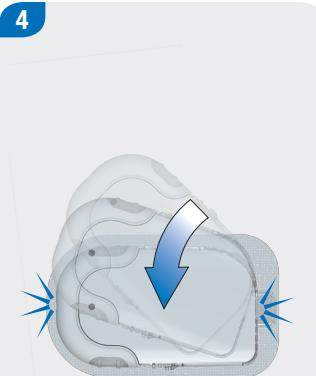
After one eighth turn (approx. 45 degrees), the micropump clicks into the front and rear hooks on the pump holder.
