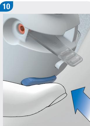
Press the blue release button to insert the cannula under the skin.
