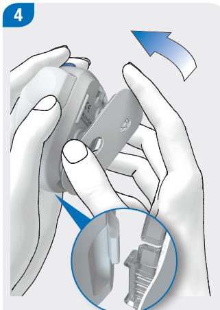
Attach the hook on the pump holder to the underside of the insertion device.
