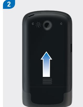
Open the battery compartment by pushing the battery door up in the direction of the arrow.
