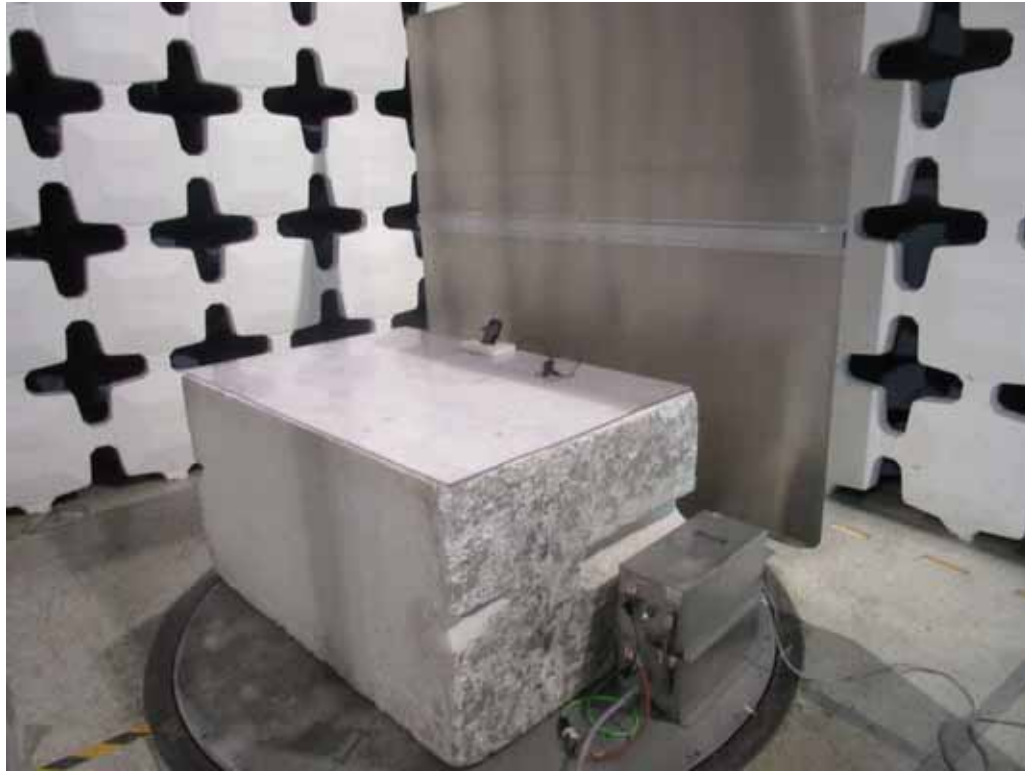
Test Setup for Conducted Emissions
