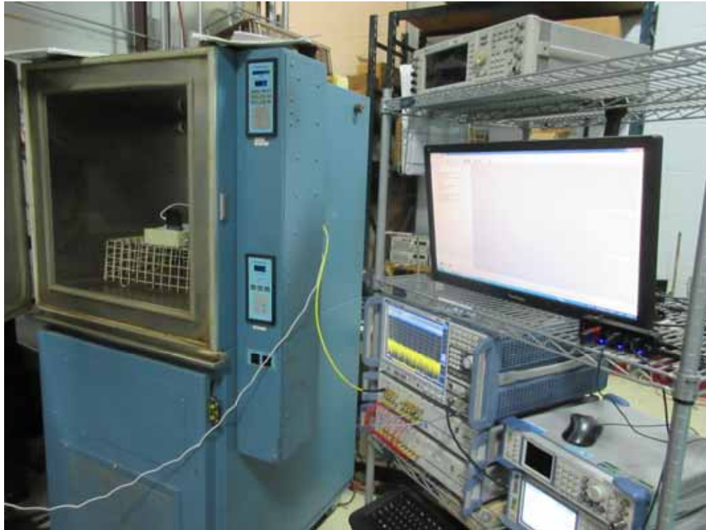
Test Setup for Antenna Conducted Emissions Tests
