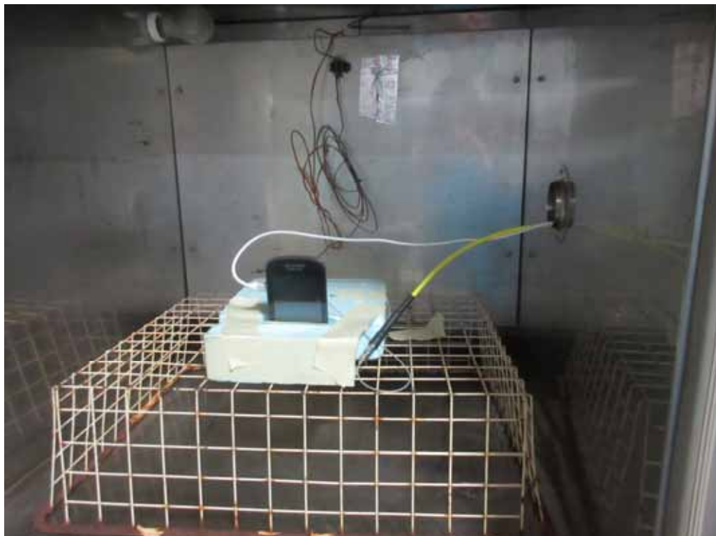
Test Setup for Antenna Conducted Emissions Tests
