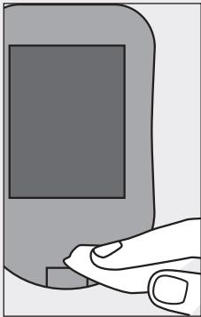
Turn the meter off and wipe the entire meter surface with a Super Sani Cloth. Carefully wipe **around** the test strip slot and other openings. Make sure that no liquid enters any slot or opening.
