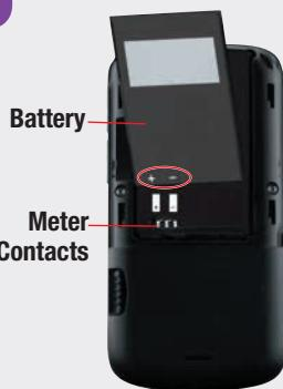
Align the new battery by placing the (+) (-) end as shown.
