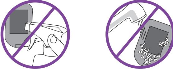
**Failure to follow these instructions will damage the meter and stop it from working properly.**
