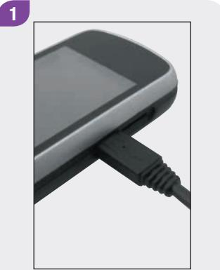
Plug the small end of the USB cable into the meter.
