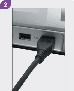
Plug the large end of the USB cable into an available USB port on the PC.
