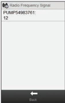
The names of the radio frequency devices with the radio frequency signal strength of each are displayed.
