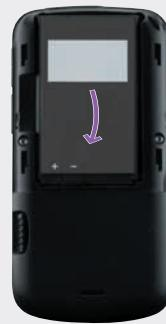
Slide the (+) (-) end of the battery against the meter contacts. Press battery into meter.
