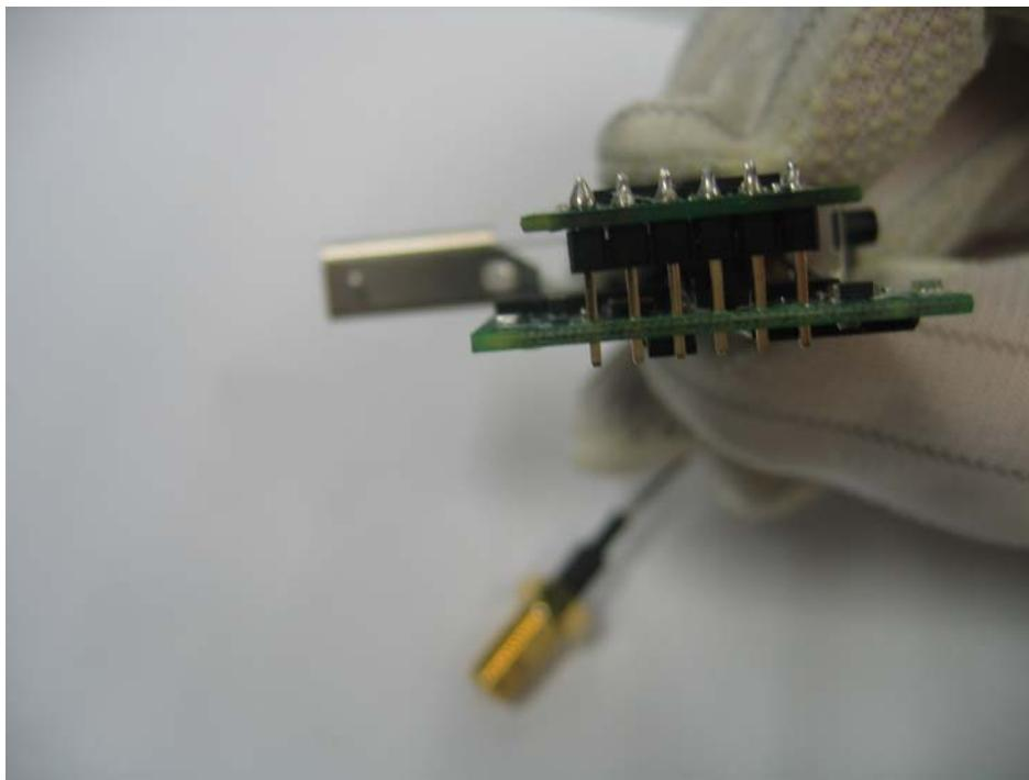
4. Make sure the module's pin connector come out on back ground of main board about 1mm and then fix it by welding.
