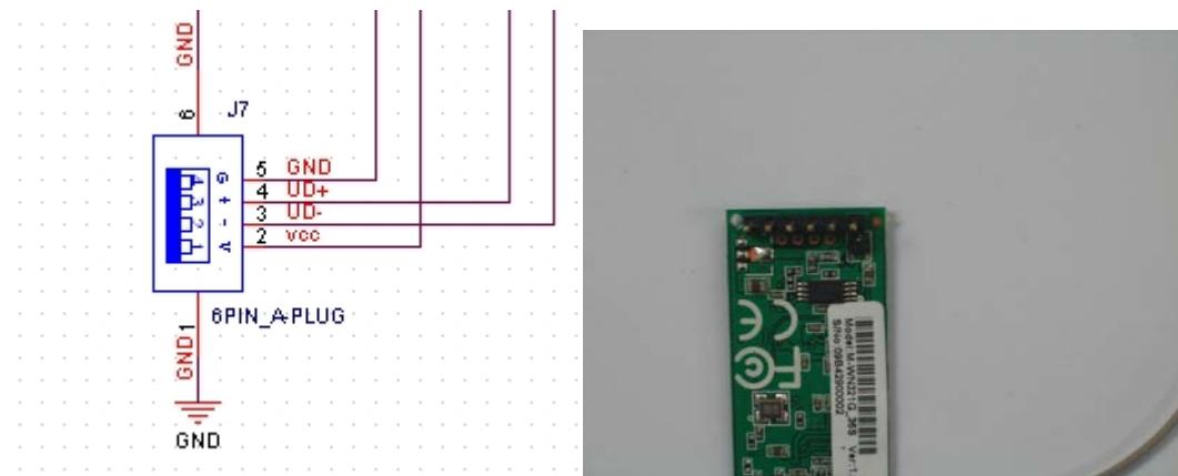
2. For using the module into your device, you should make sure the device has the same pin hole and the right pin definition. Below is the sample of wireless print server's main board. This print server has six pin holes and it is designed according to standard USB2.0. the pin hole's turn is from left to right.
