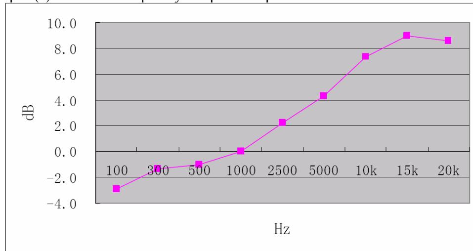
0dB=12mV at 1kHz (20% of the maximum rated system deviation).
