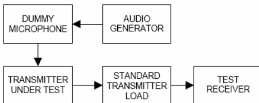
Test at five different modulating frequencies (100Hz, 300Hz, 500Hz, 1 KHz, 2.5 KHz, 5kHz), the output level of the audio generator was varied and the FM deviation level was recorded. Positive peak deviation
