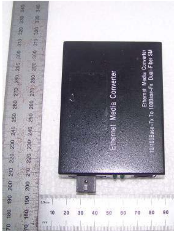
Sample with SFB transceiver
