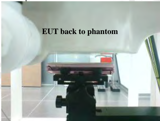
Fig.6 Body worn- EUT back to flat phantom and distance between flat phantom and mobile phone is 1.5 cm
