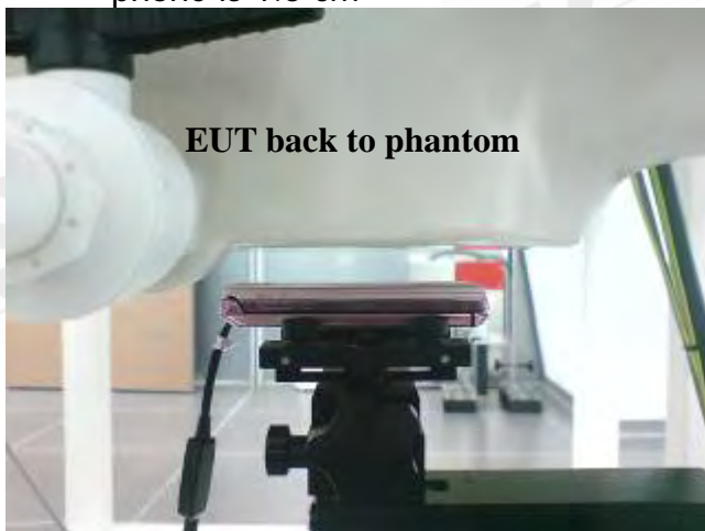
Fig.7 Body worn- EUT back to flat phantom and distance between flat phantom and mobile phone is 1.5 cm with headset
