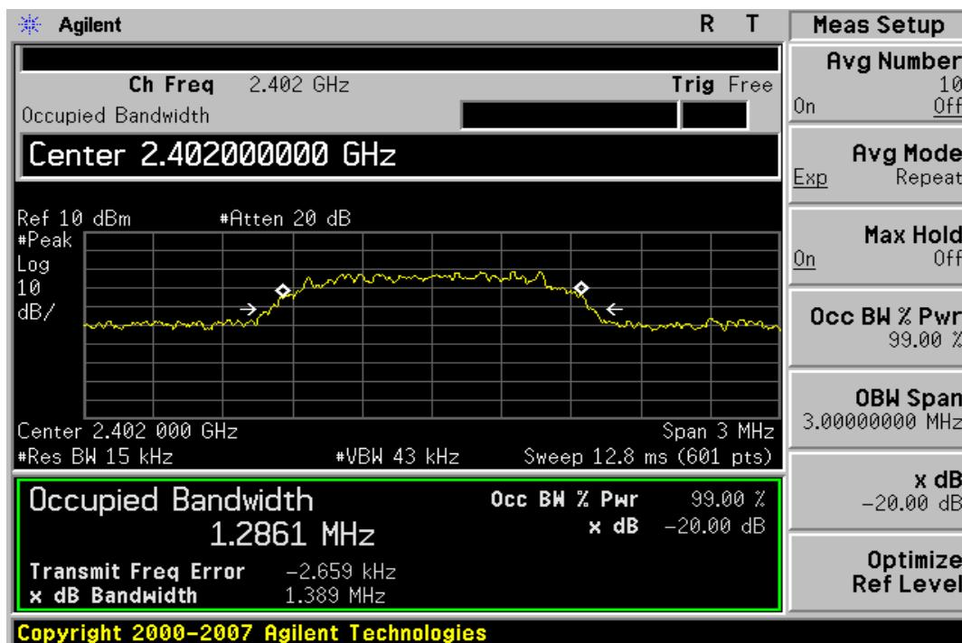
**20dB Bandwidth Test Data CH-Mid**
