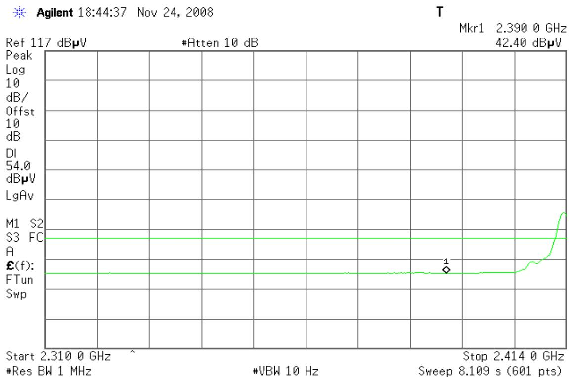
**Band Edges (CH High)****Detector mode: Peak****Polarity: Vertical**
