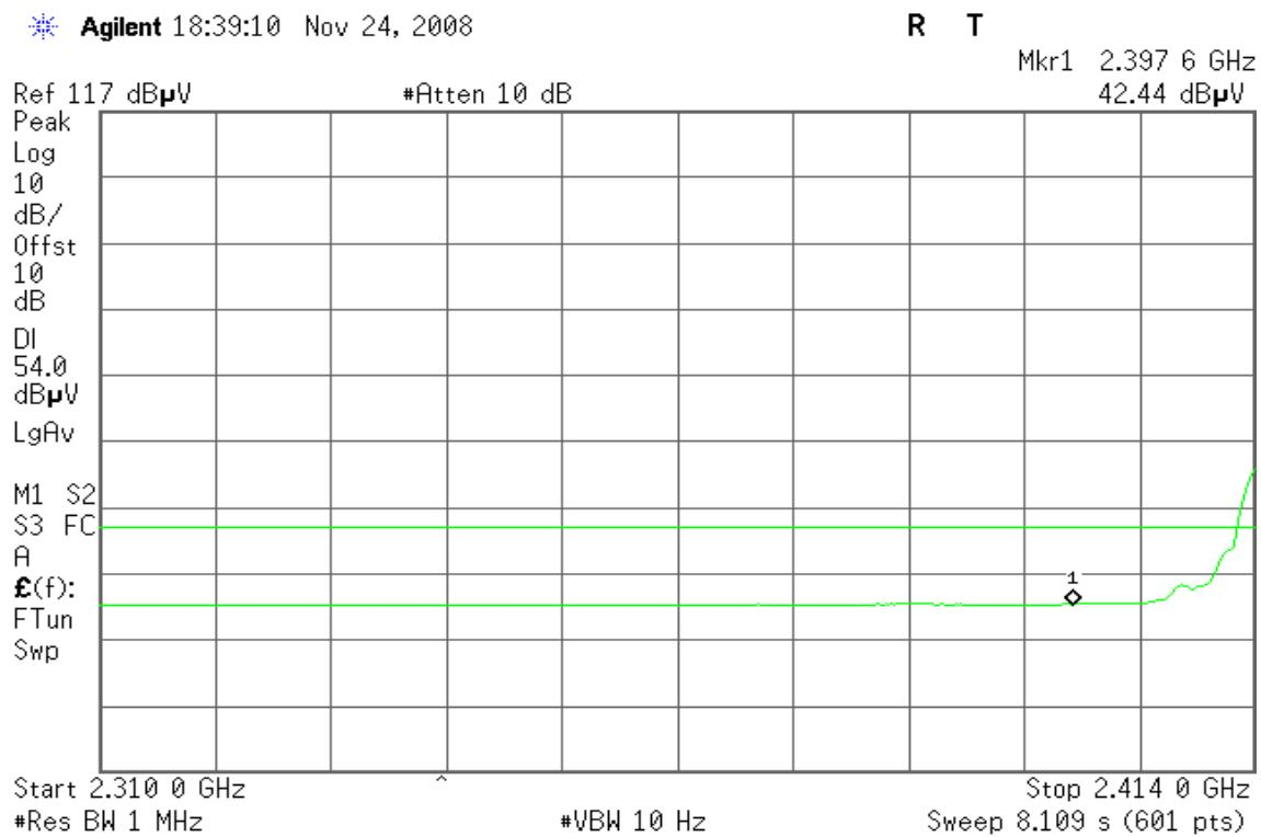
**Detector mode: Peak****Polarity: Horizontal**
