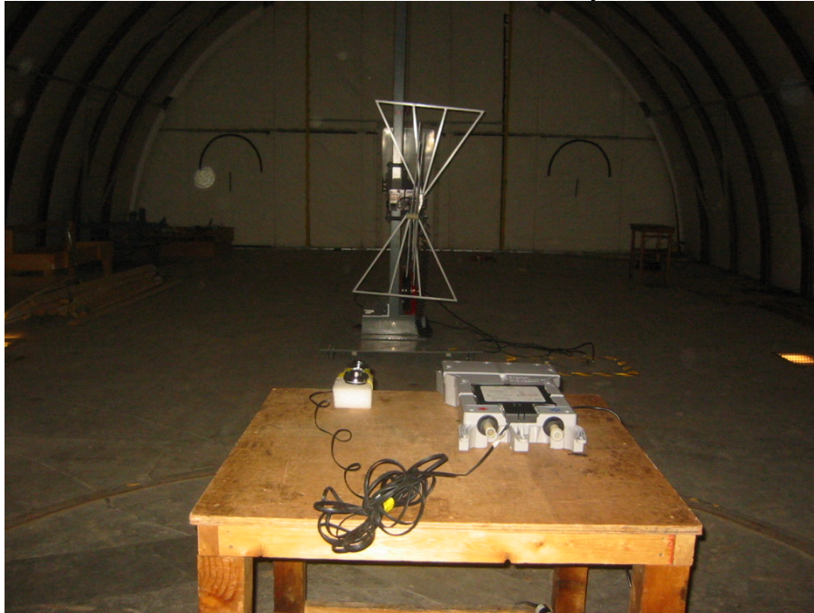
Controller Radiated Emissions Setup Photo
