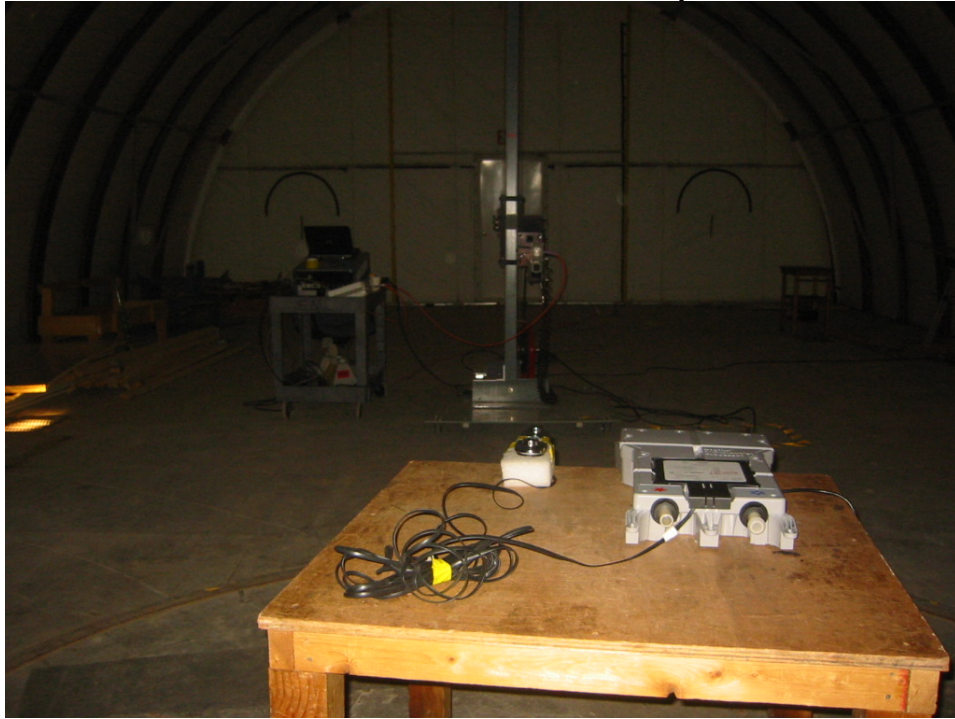
Controller Radiated Emissions Setup Photo
