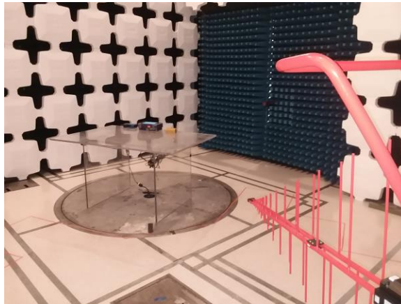
Figure 2: Radiated Emissions Test Setup Below 1GHz
