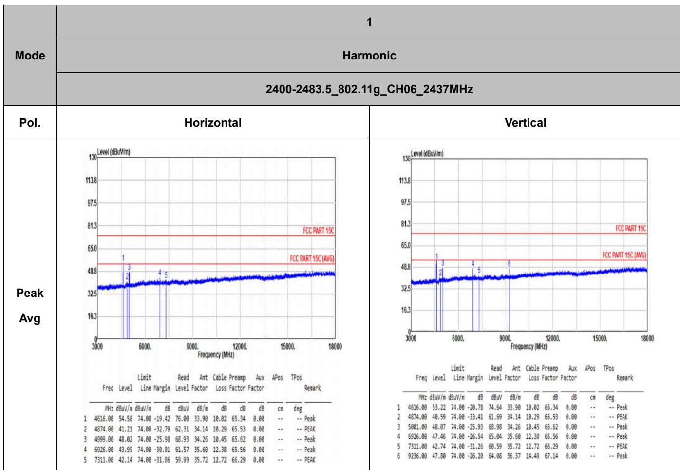
Note: #1/4 of Horizontal and #1/4/6 of Vertical are from WWAN bands which are Harmonics. Please refer to Table 2, the Peak levels meet for limit.
