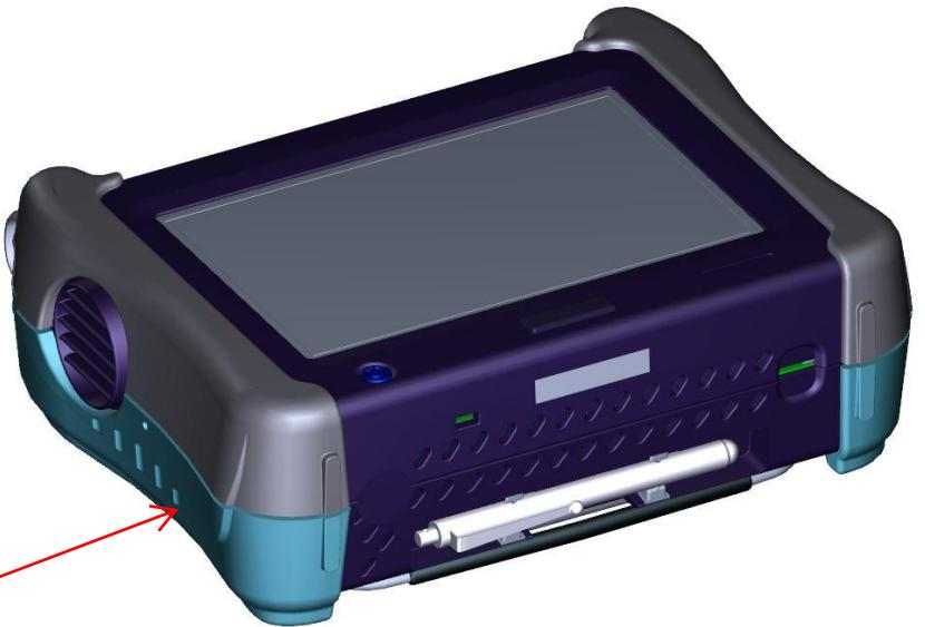
Radio module and antenna are located in this corner of the device.
