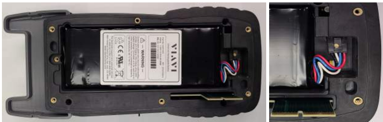
Figure B-6 Battery Cables and Release Clip
