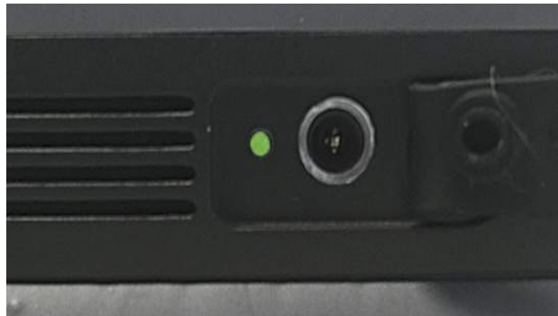
Figure 1-7 CX100 Battery LED
