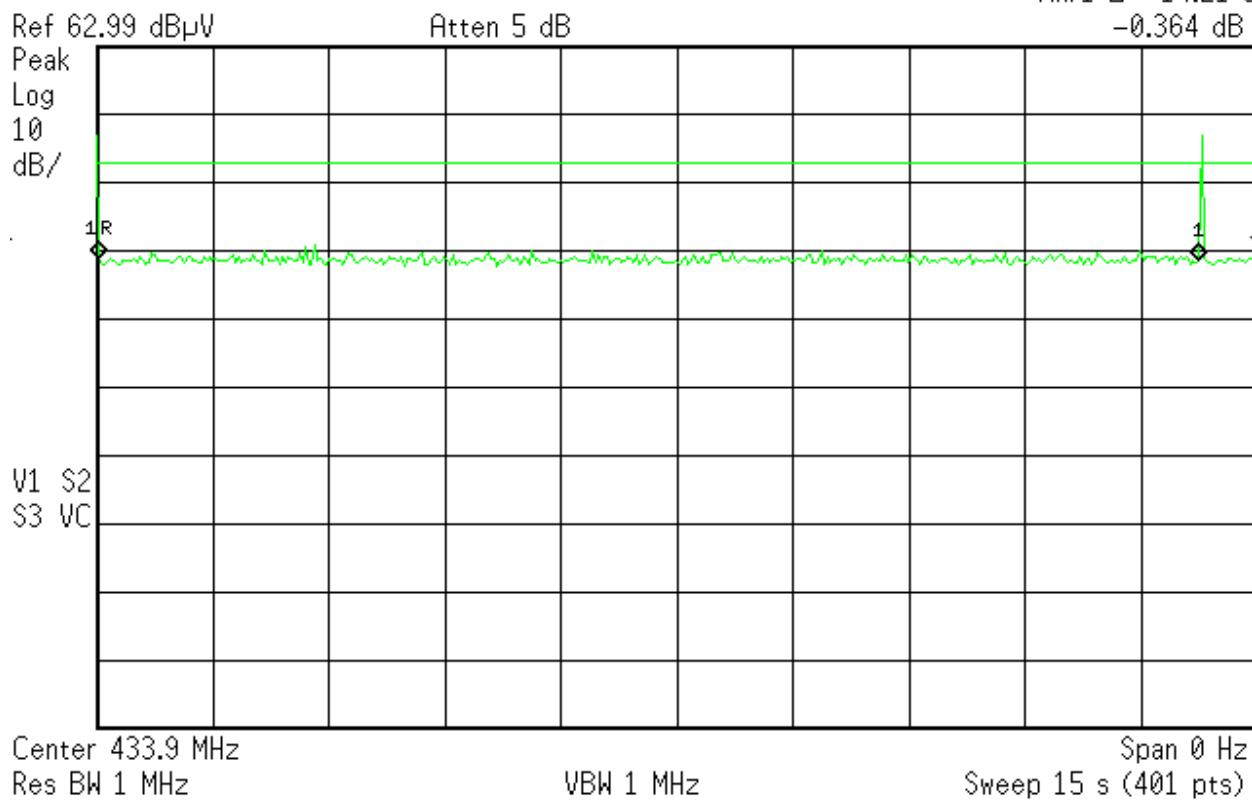
The worst case duty cycle is represented by the two analyzer plots immediately above.
