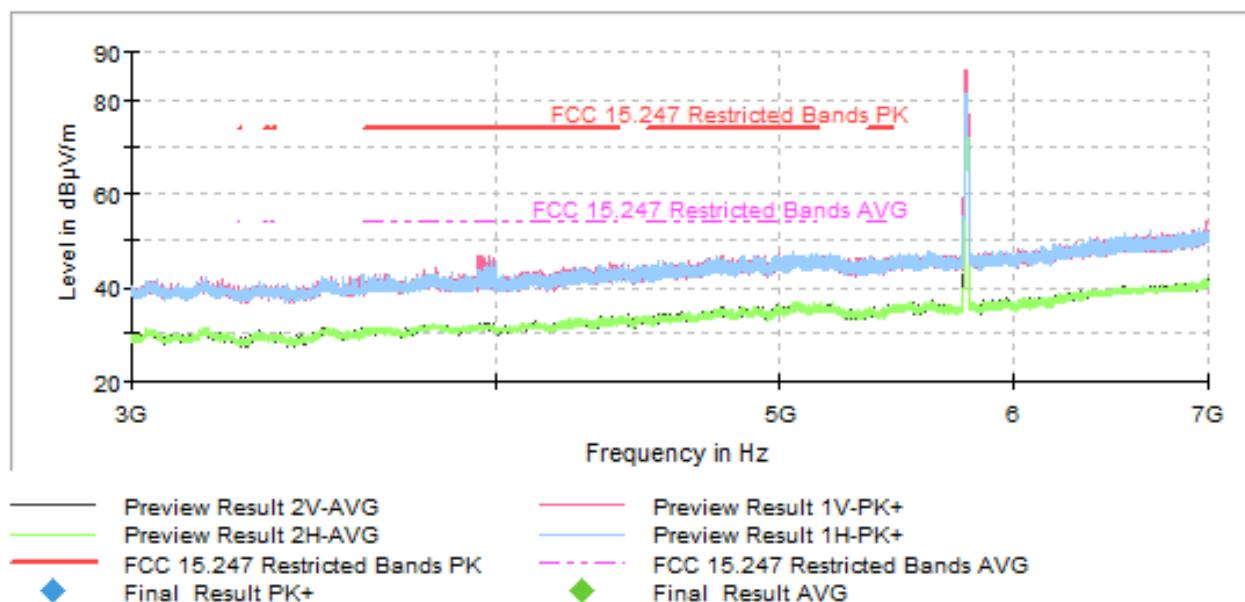
The peak above the highest limit is the WLAN 5 GHz carrier frequency.
