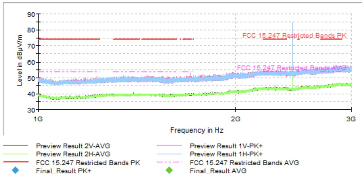
The peak above the highest limit is the Bluetooth EDR carrier frequency.
