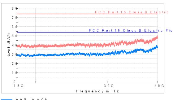
A V G \_ M A X H P K + \_ M A X H F C C P a rt 1 5 FCC Part 15 Class B Electric Field Strength PK FCC Part 15 Class B Electric Field Strength QP+AV
