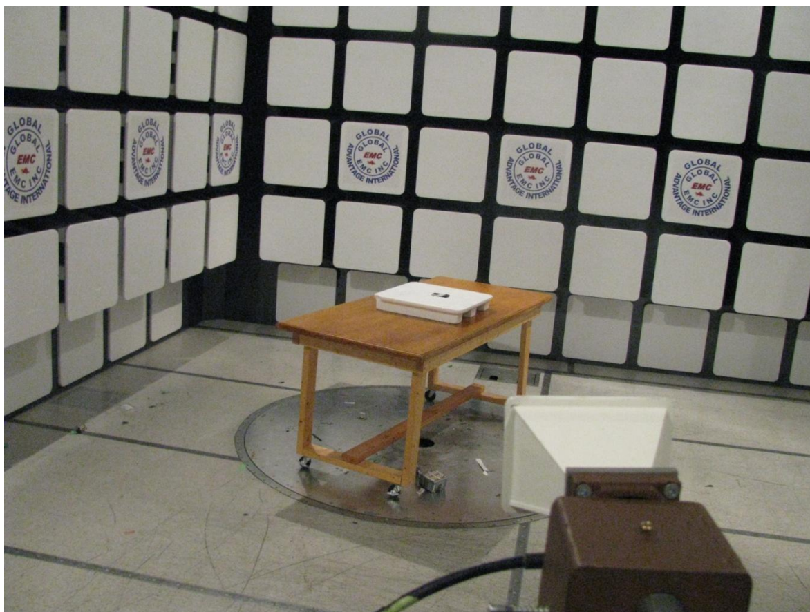
Figure 1 – Radiated emission setup
