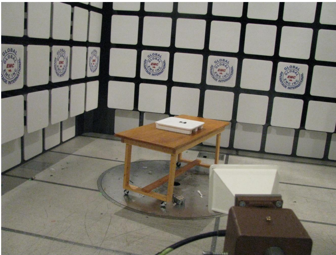
Figure 1 – Radiated emission setup
