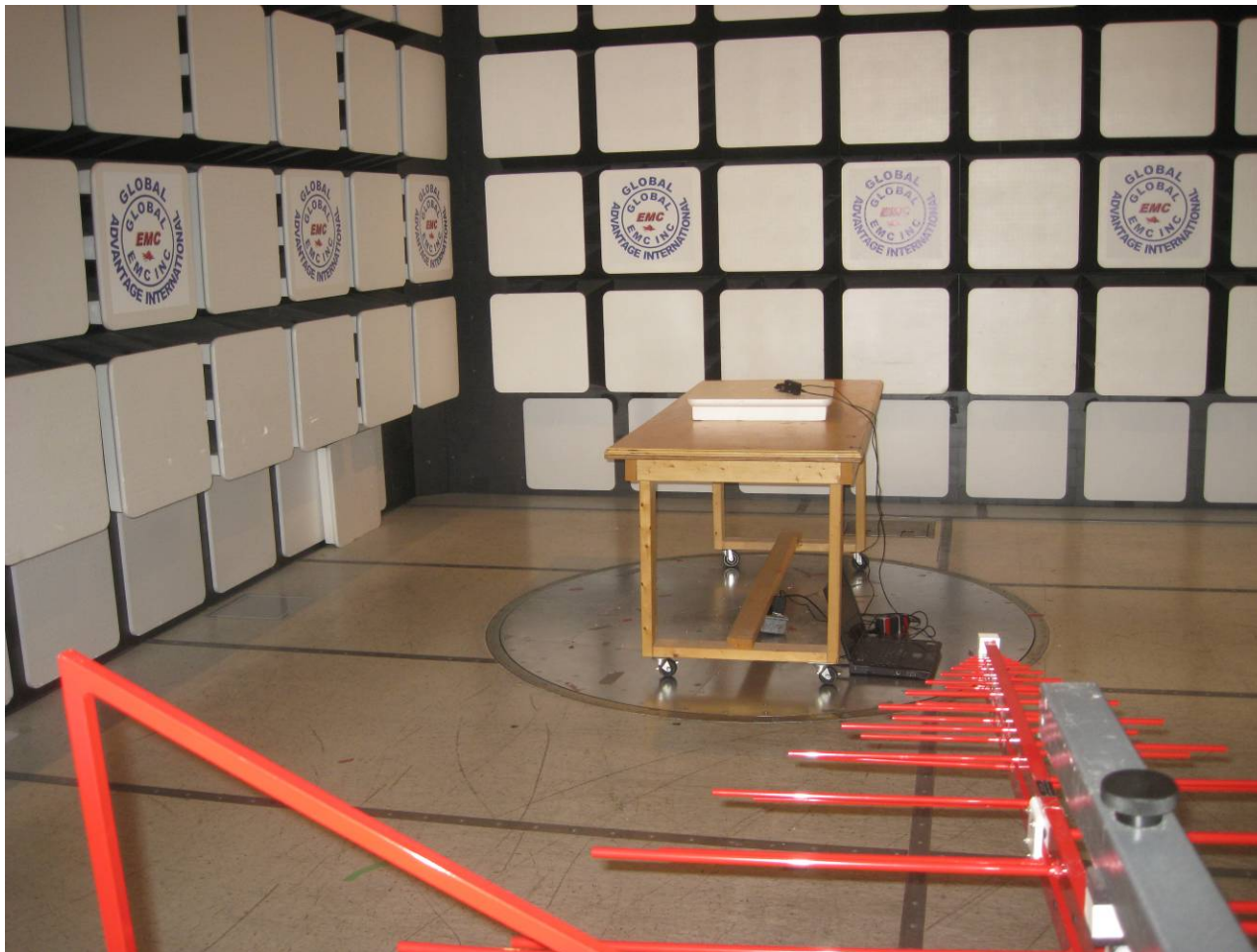
Radiated Emissions 2 – Setup
