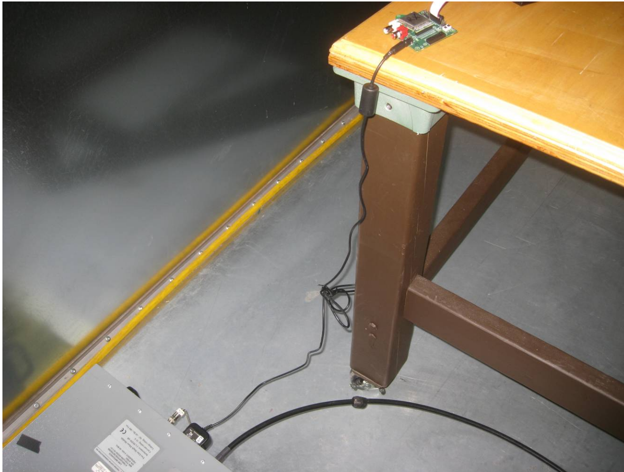
Power Line Conducted Emissions Setup 2
