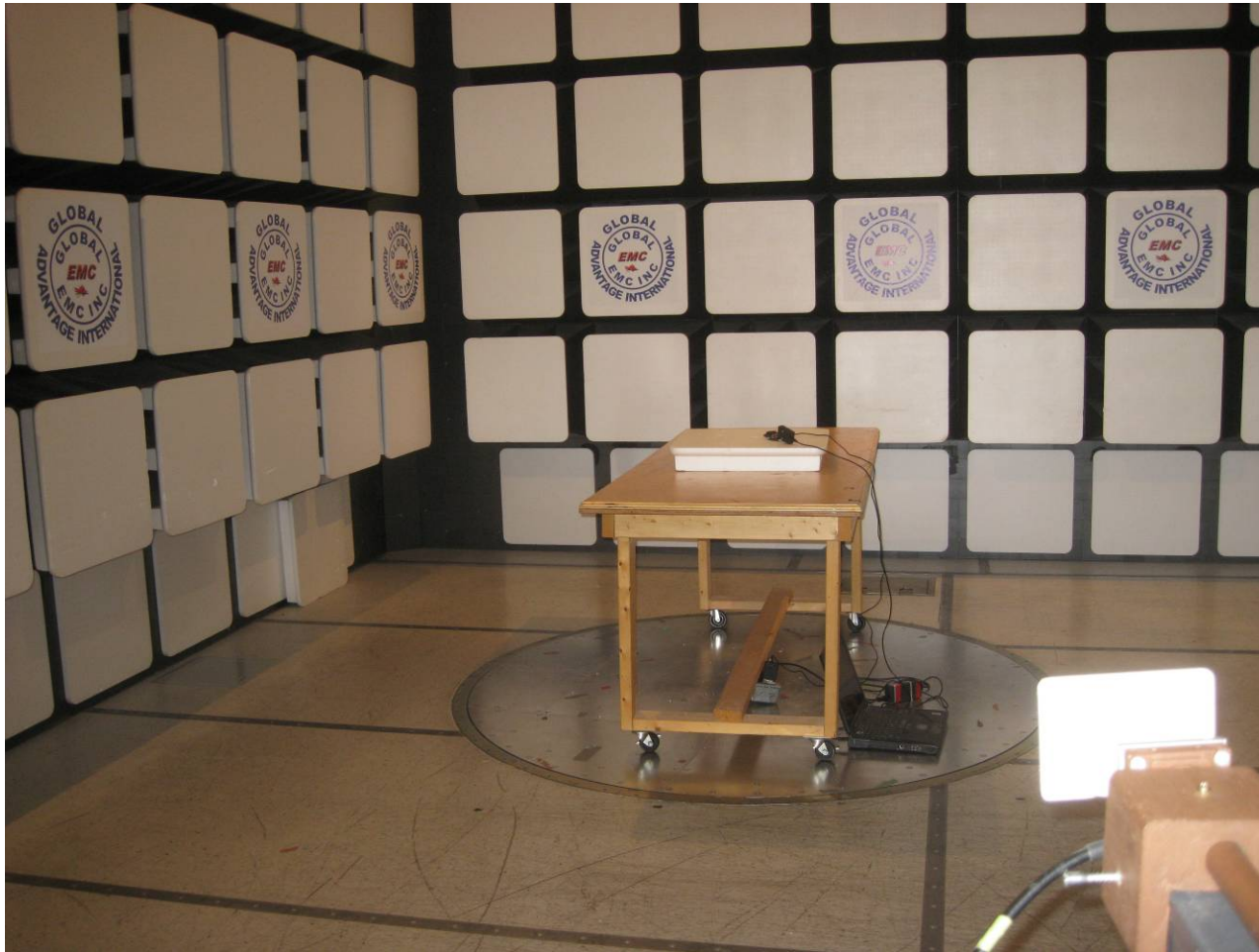
Radiated Emissions – Setup
