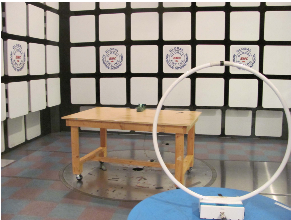
Illustration 2: Radiated emission setup - photo 2
