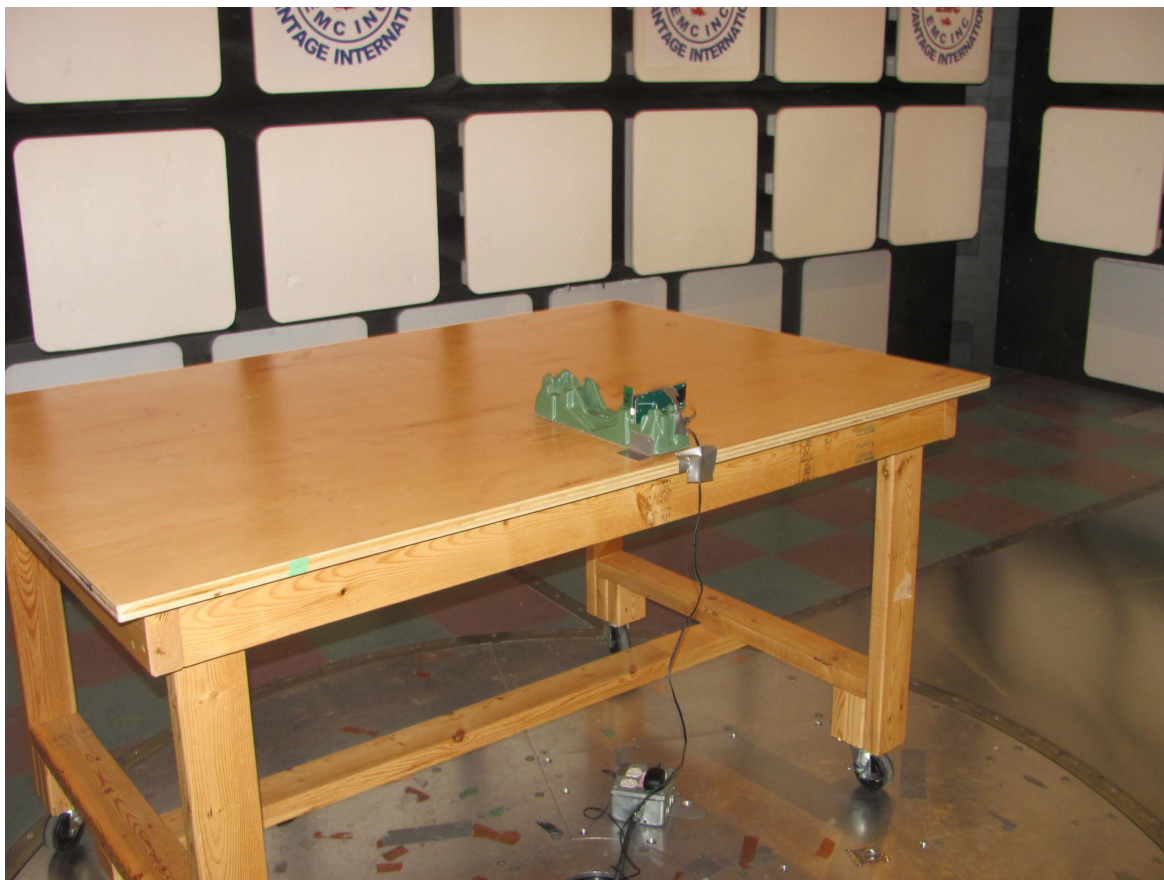
Illustration 1: Radiated emission setup – photo 1
