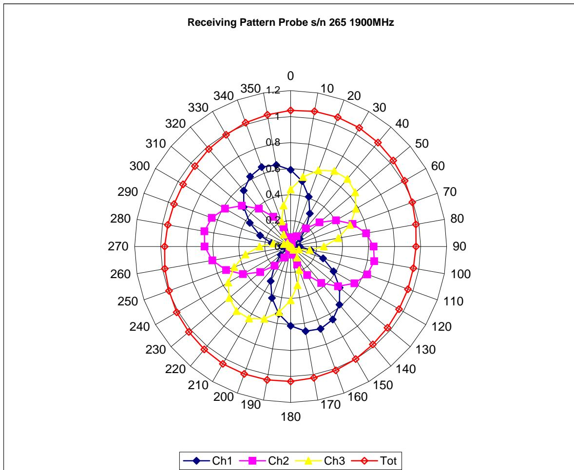
**Isotropy Error 1900 MHz (Air)**
