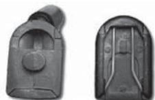
**Camlock mount** - Generally standard on vehicles manufactured outside of the United States. This style of mirror must be removed by turning the mirror 90 degrees so that it is perpendicular to the dash, and pulling down on the mirror.
