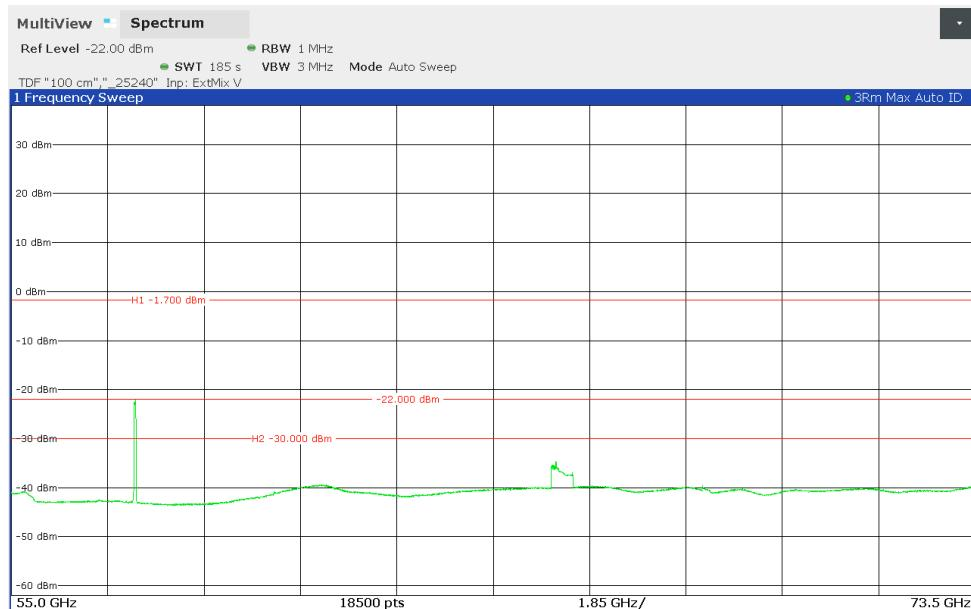
Signal ID function is used. The diagram shows image signals and mixer products. The real input signal is shown, only when USB and LSD traces have the same position on the frequency axis. Emissions from 57.340 GHz to 57.402 GHz and 65.359 GHz to 65.781 GHz are a products caused by the harmonic mixer, please refer the plot below for the signal identification.
