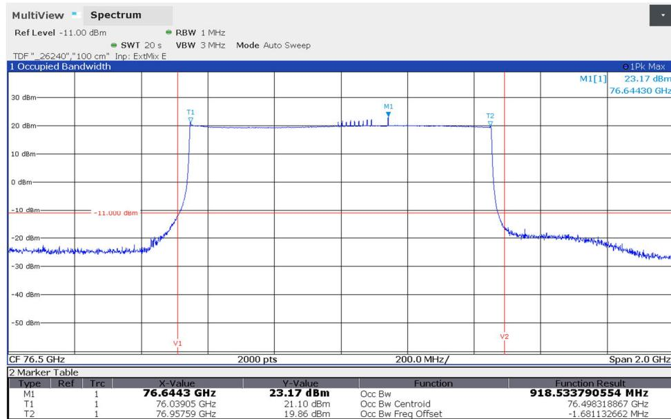
201003\_6d.png: Maximum effective radiated isotropically peak power and occupied bandwidth (variant 4):
