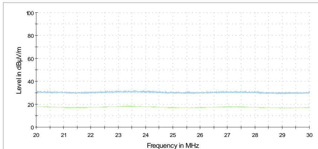
201003\_20M-30M\_V4: Radiated spurious emissions from 20 MHz to 30 MHz (variant 4):
