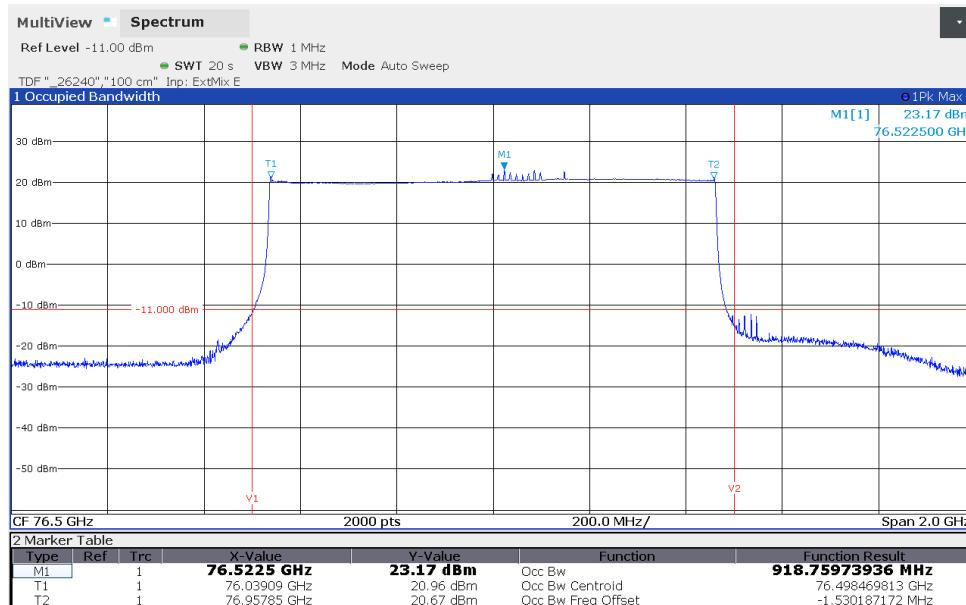
201003\_46d.png: Maximum effective radiated isotropically peak power and occupied bandwidth (variant 4):
