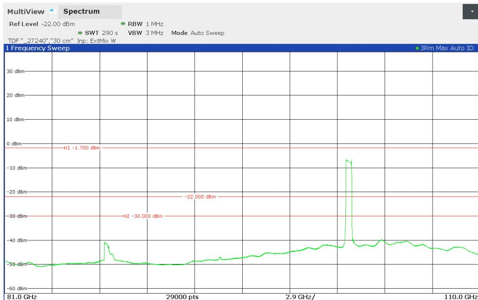
Signal ID function is used. The diagram shows image signals and mixer products. The real input signal is shown, only when USB and LSD traces have the same position on the frequency axis. Emissions from 87.083 GHz to 87.684 GHz and 101.717 GHz to 102.250 GHz are a products caused by the harmonic mixer, please refer the plot below for the signal identification.
