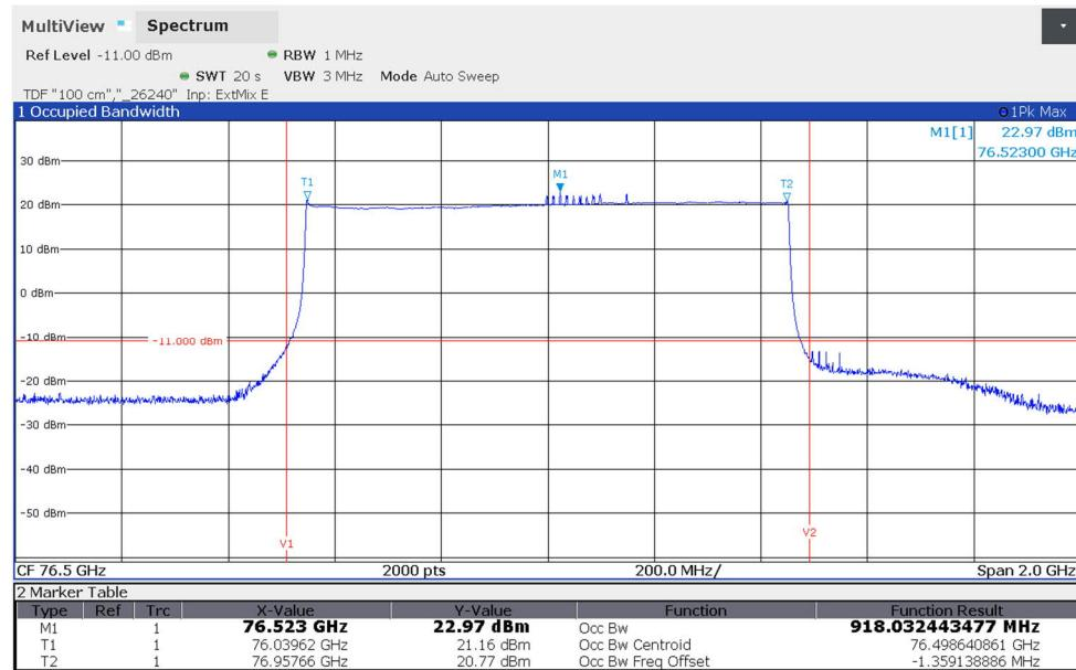
201003\_46b.png: Maximum effective radiated isotropically peak power and occupied bandwidth (variant 2):
