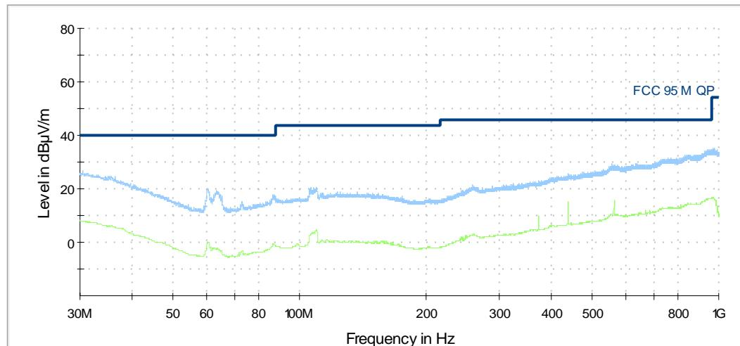
201003\_30M-1G\_V4: Radiated spurious emissions from 30 MHz to 1 GHz (variant 4):
