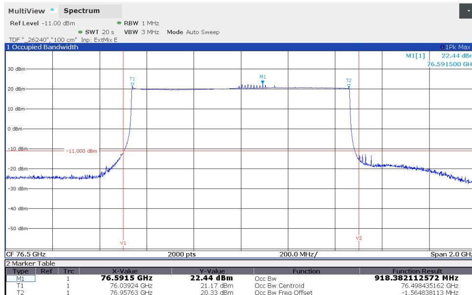
201003\_44d.png: Maximum effective radiated isotropically peak power and occupied bandwidth (variant 4):
