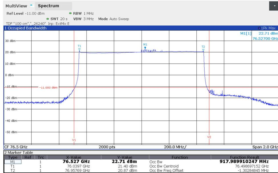
201003\_44b.png: Maximum effective radiated isotropically peak power and occupied bandwidth (variant 2):
