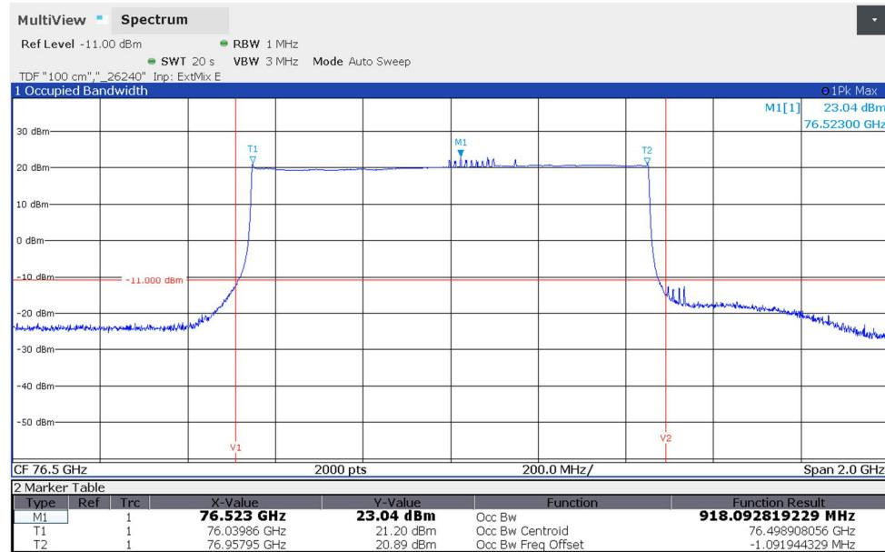
201003\_6b.png: Maximum effective radiated isotropically peak power and occupied bandwidth (variant 2):
