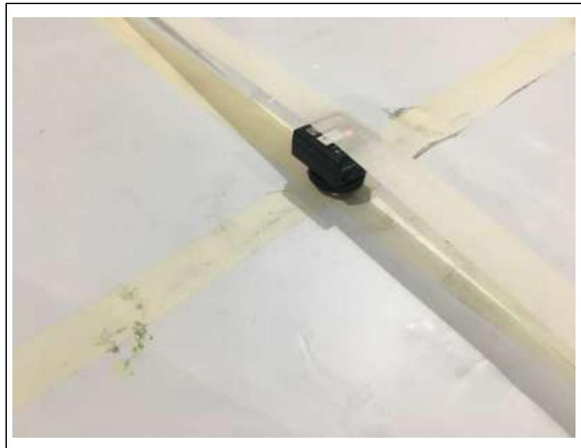
***2. Photo of Radiated Spurious Emission Test (Below 1 GHz)***
