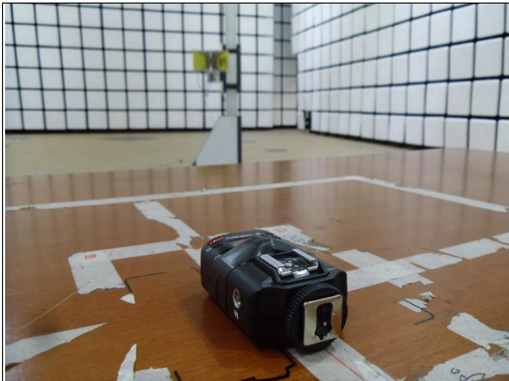
Photo of Field Strength & Spurious Emission Test(Above 1 GHz)
