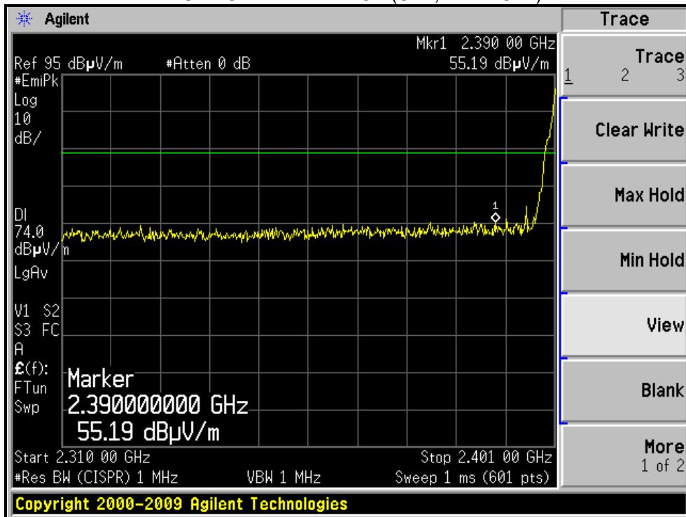
\* The average value of fundamental frequency is: Average = Peak value +  $20\log(\text{Duty cycle})$ . And it meets the requirement of limit.
