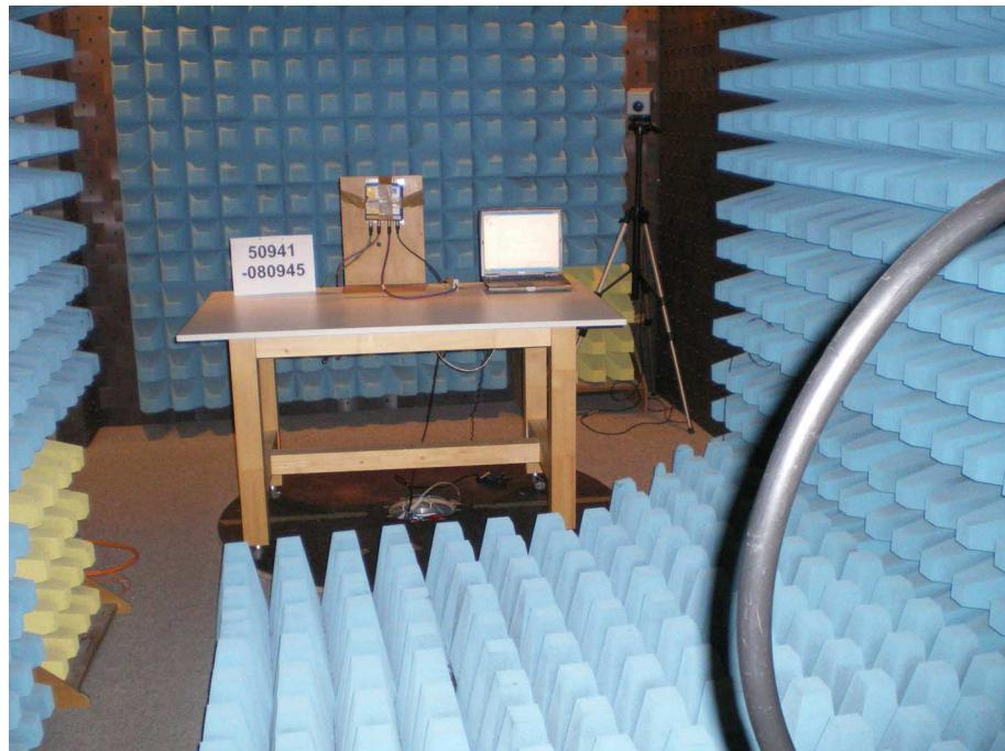
**Test setup for radiated emission measurement
