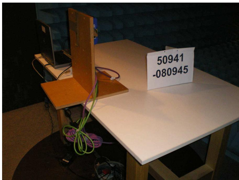
**Test setup for radiated emission measurement
