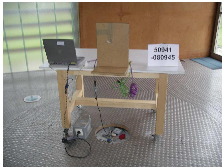
**Test setup for radiated emission measurement
