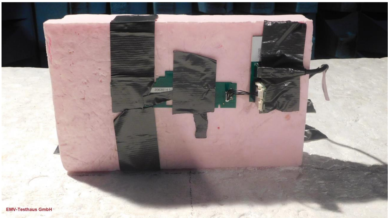
Picture 34: EUT-position 2 - PCB antenna set 2063514:5171
