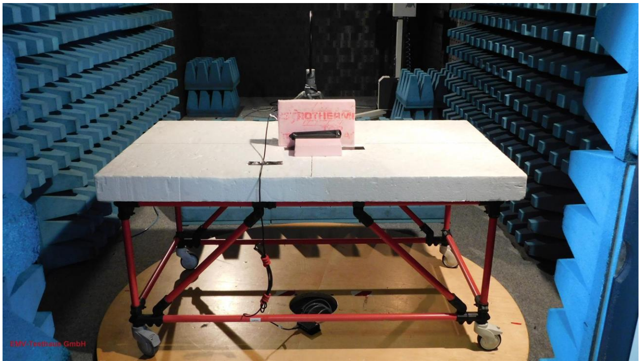
Picture 3: CDC, test setup radiated emission test 9 kHz -30 MHz - PCB antenna 2009168:4834 (front view)
