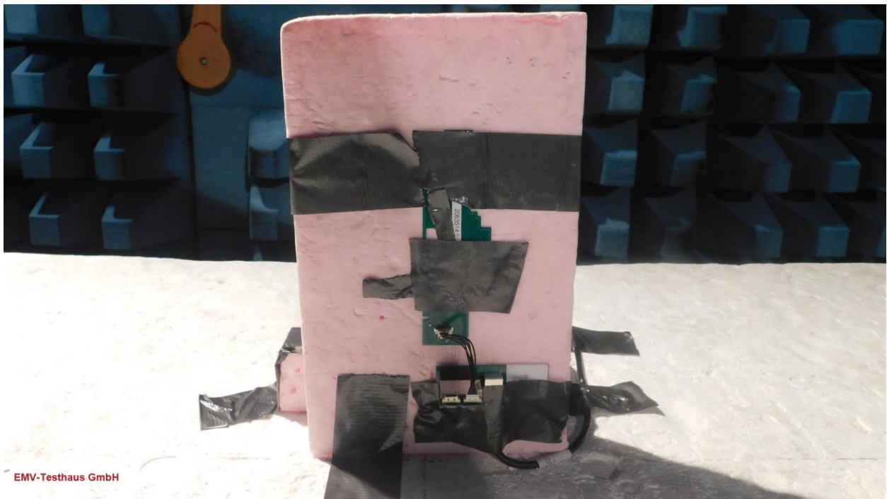
Picture 33: EUT-position 1 - PCB antenna set 2063514:5171
