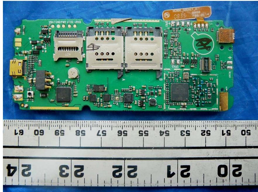
**14.12 EUT – Main Board Assembly (with LCD and keyboard) Top View**
