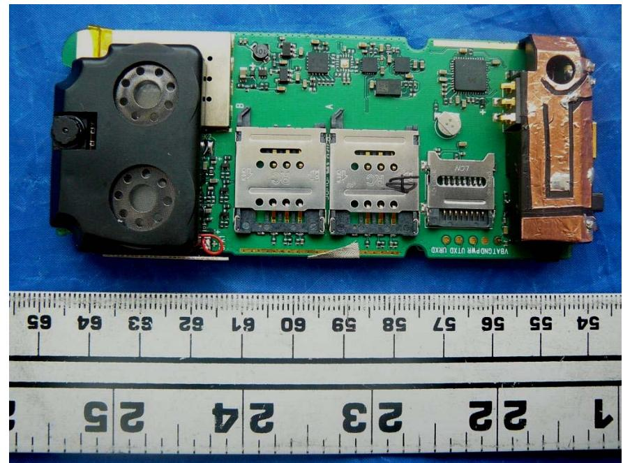
**14.11 EUT – Main Board Assembly (without Antenna and RF Sheilding) Bottom View**
