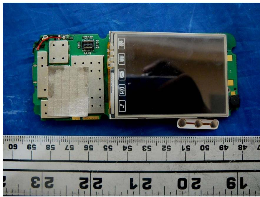
**14.15 EUT – Main Board Assembly (without keyboard) Top View 2**
