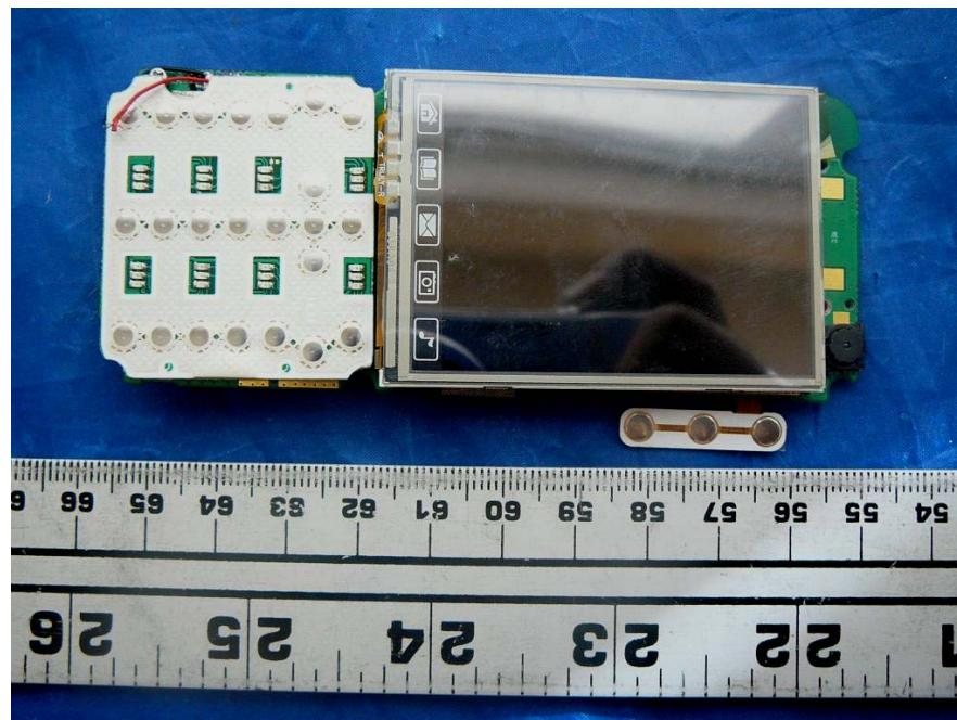
**14.13 EUT – Main Board Assembly (with LCD flip off) Top View**
