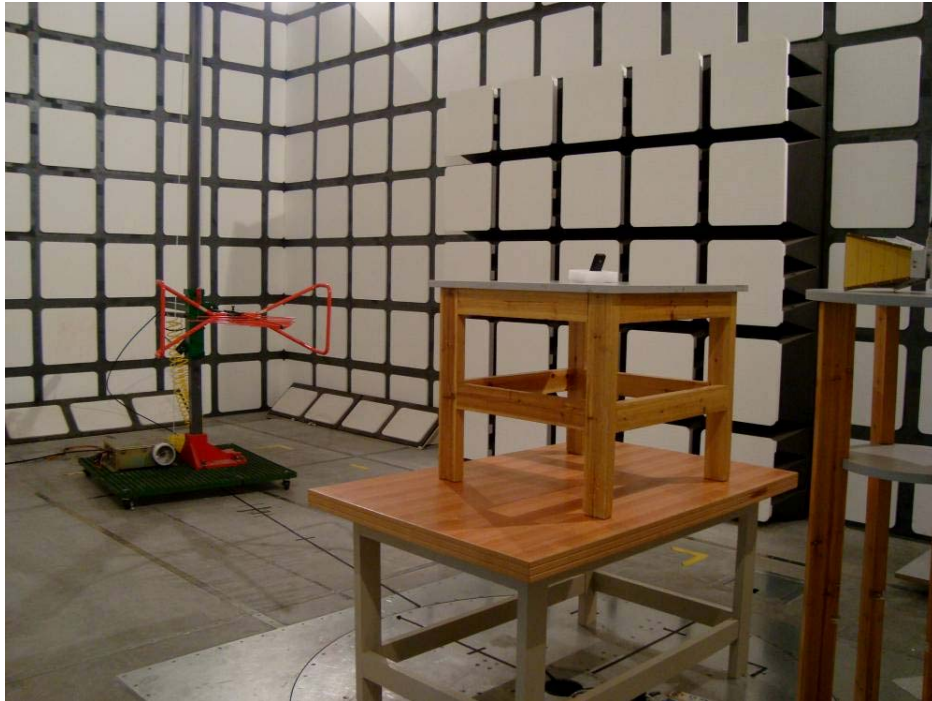
Below 1 GHz: Spurious Radiated Emissions - Rear View
