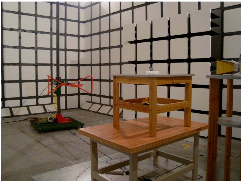
Below 1 GHz: Spurious Radiated Emissions - Rear View
